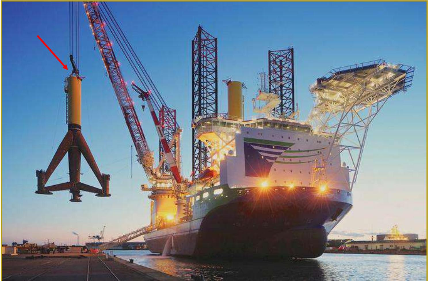
Tripod Lifting Tool SWL 950 t
