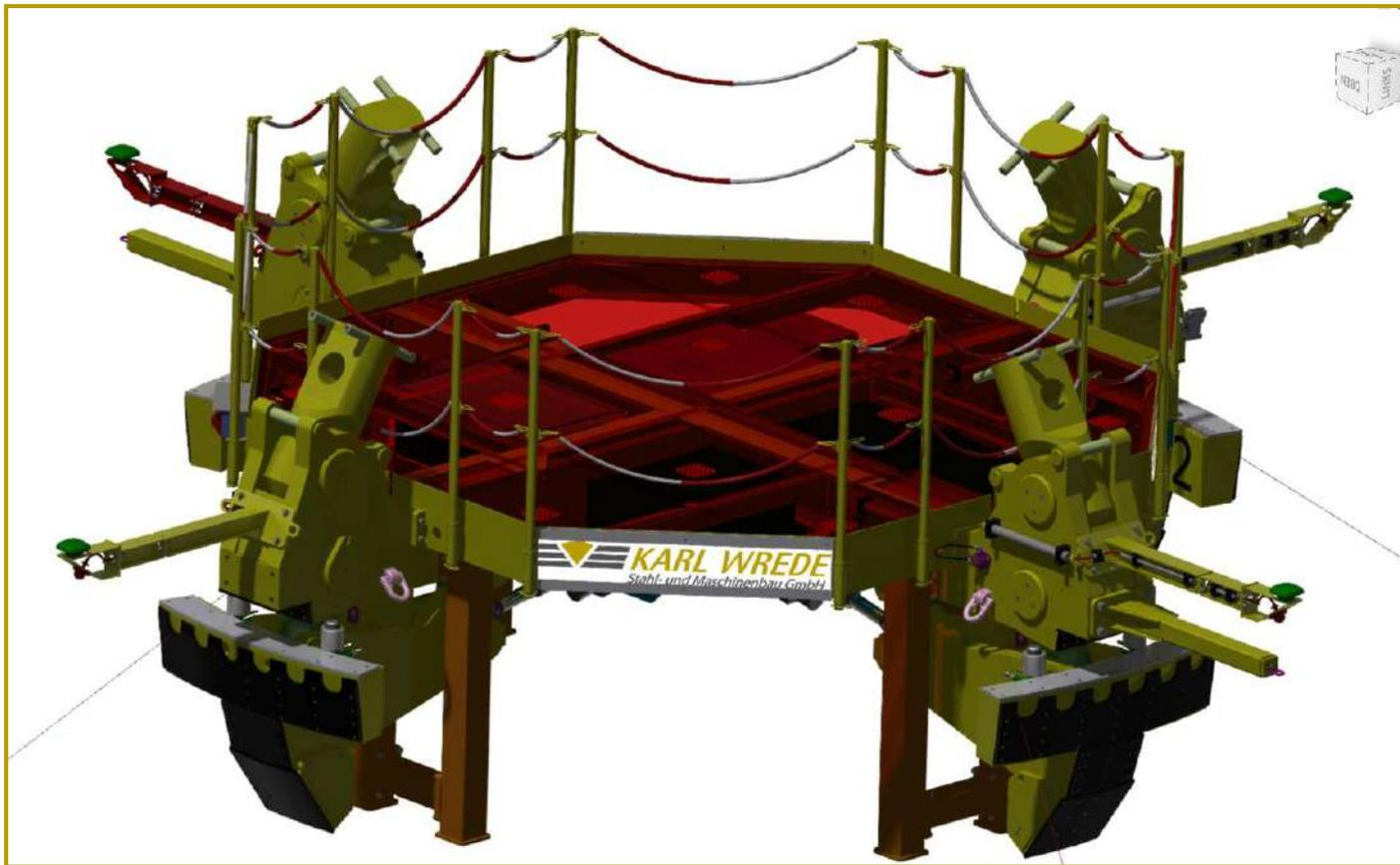
Tripod Lifting Tool SWL 950 t
