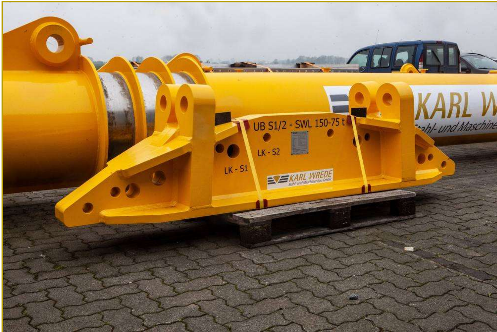
Lifting device for tower SWL 150 t
