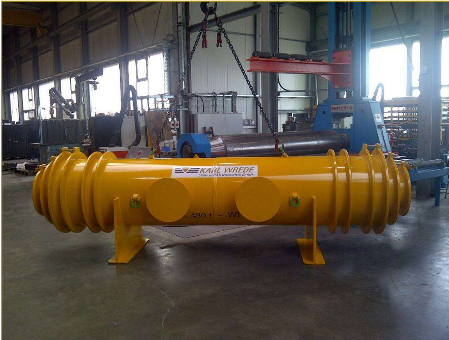
Nacelle lifting beam SWL 480 t – manual centre of gravity adjustment
