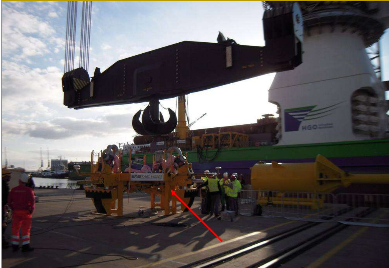
Tripod Lifting Tool SWL 950 t
