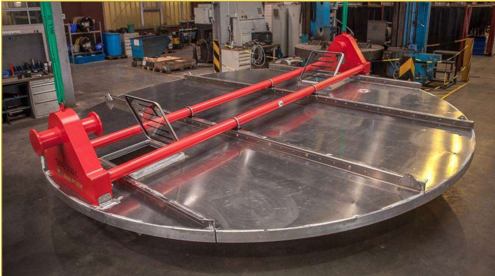
padeye transition piece SWL 200 t + cover plate - 4 MW
