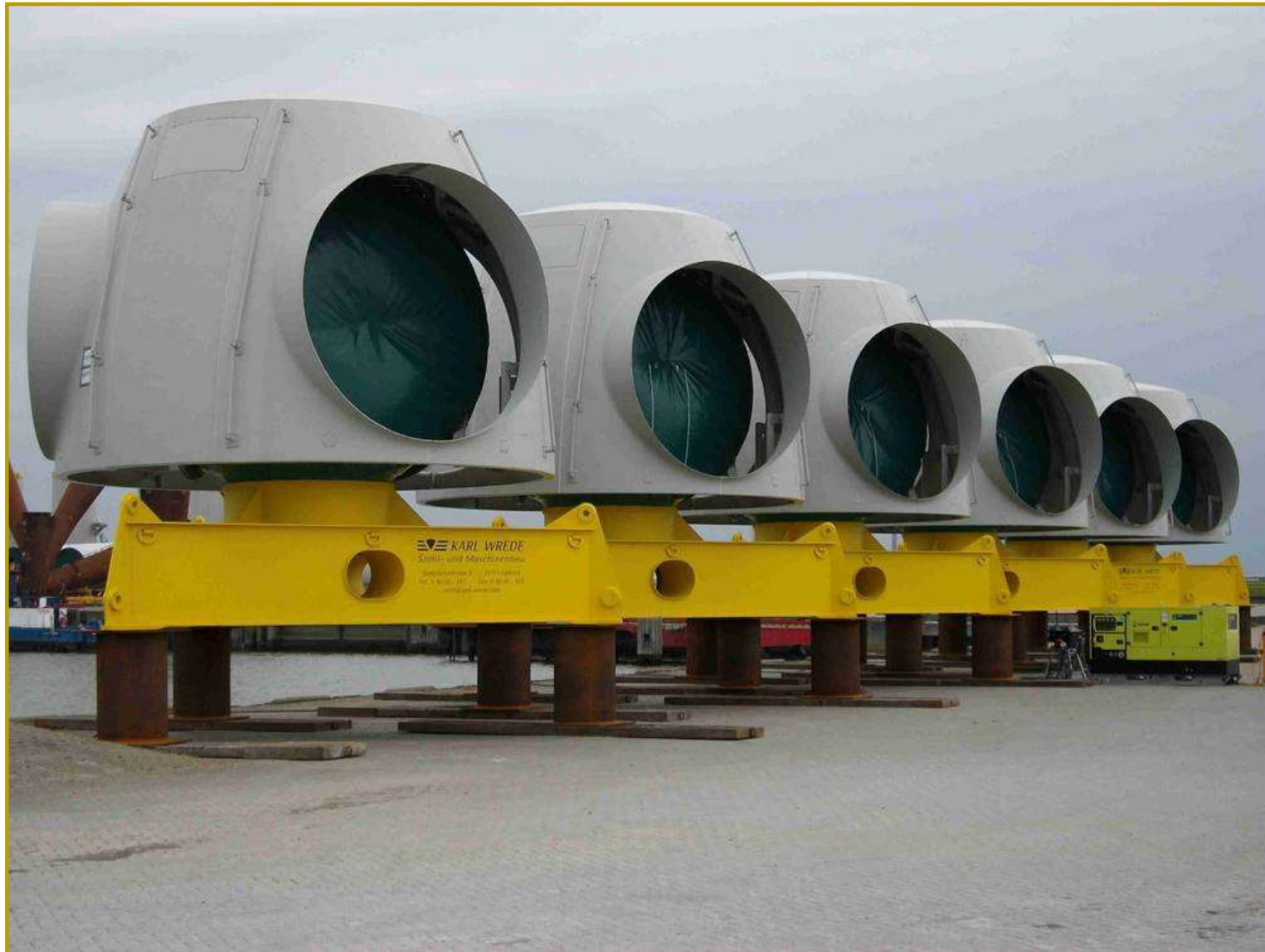
Transport frame for rotor hub 5 MW
