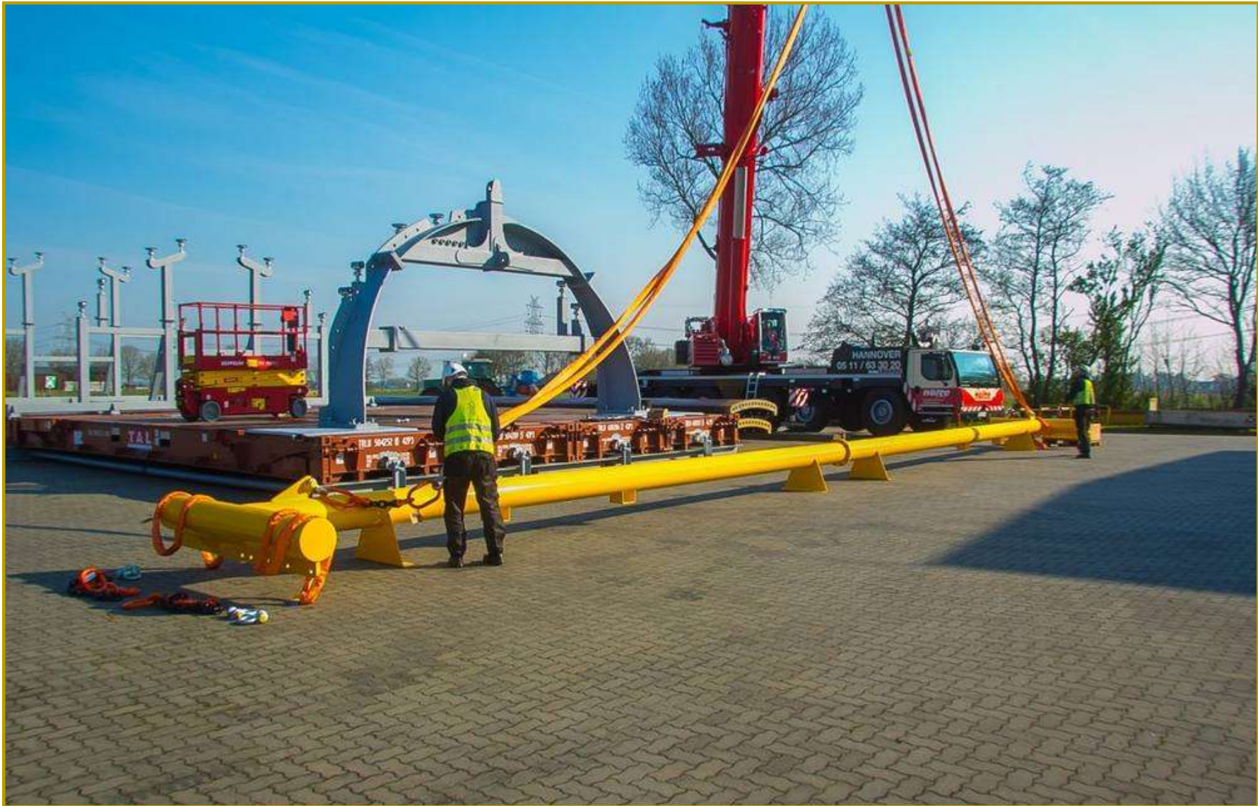
Spreader and pre-assembly device for segmented tubular steel tower
