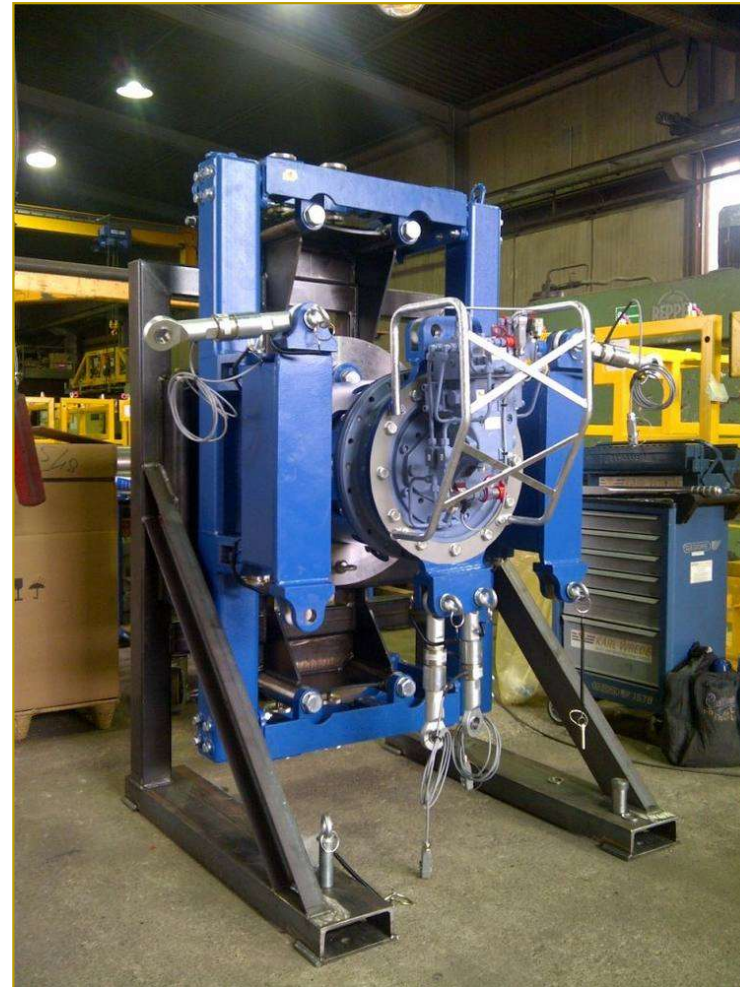
Hydraulic rotary drive system for drivetrain 6 MW offshore (single blade installation): test device
