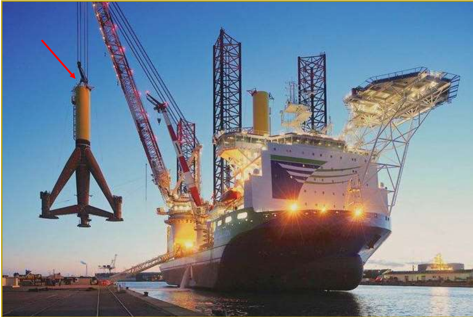
Tripod Lifting Tool SWL 950 t
