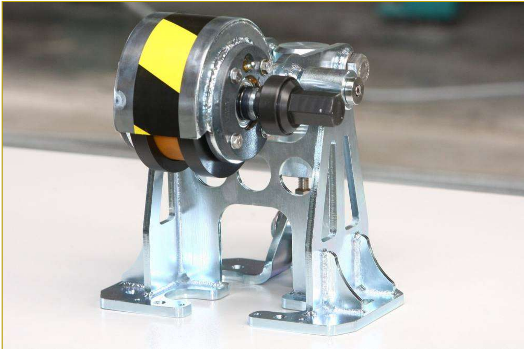
Turning device for drivetrain for service use
