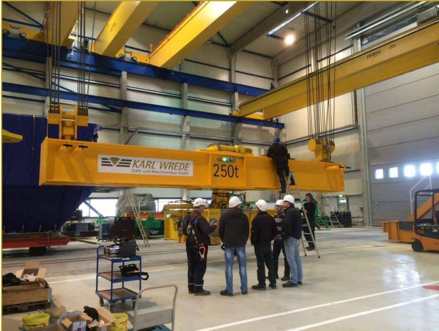
250 t assembly lifting beam combination
