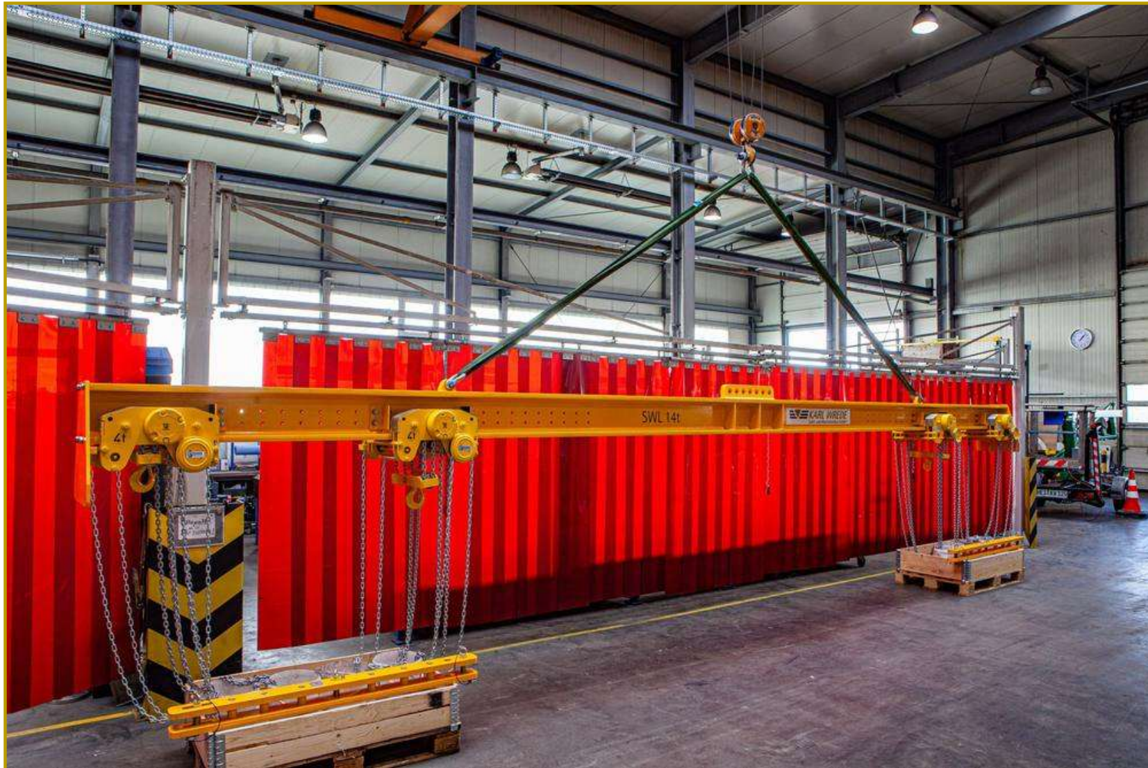
Lifting beam for transformer replacement
