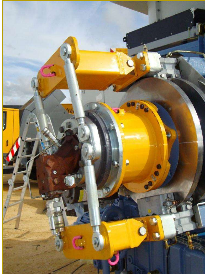
Hydraulic rotary drive system for drivetrain 3 MW (single blade installation)
