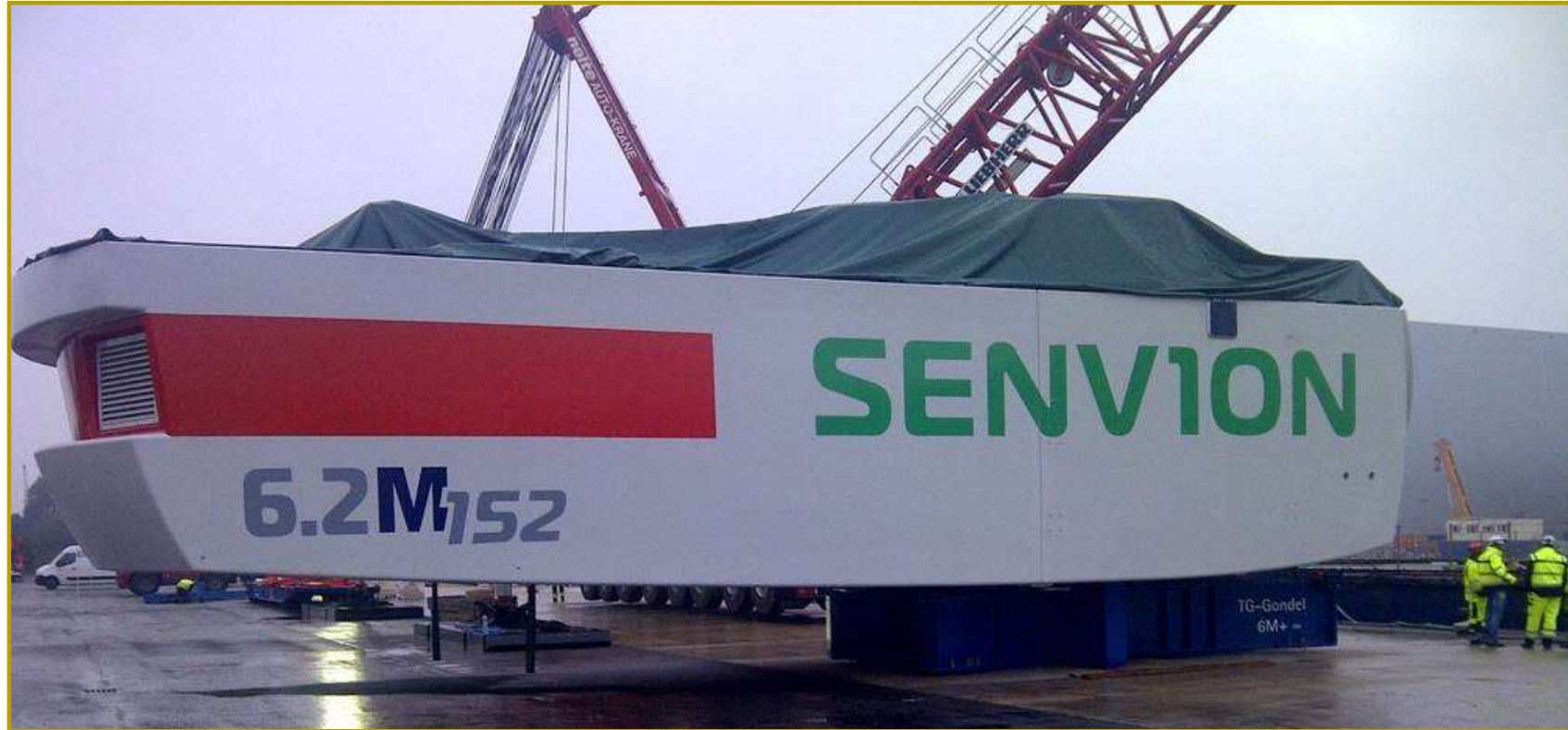
Transport frame for nacelle 6 MW
