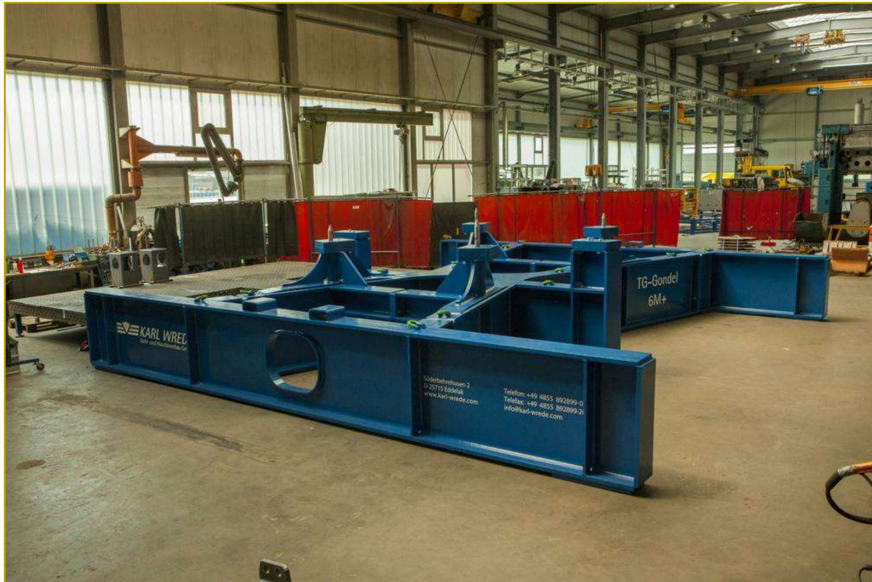
Transport frame for nacelle 6 MW
