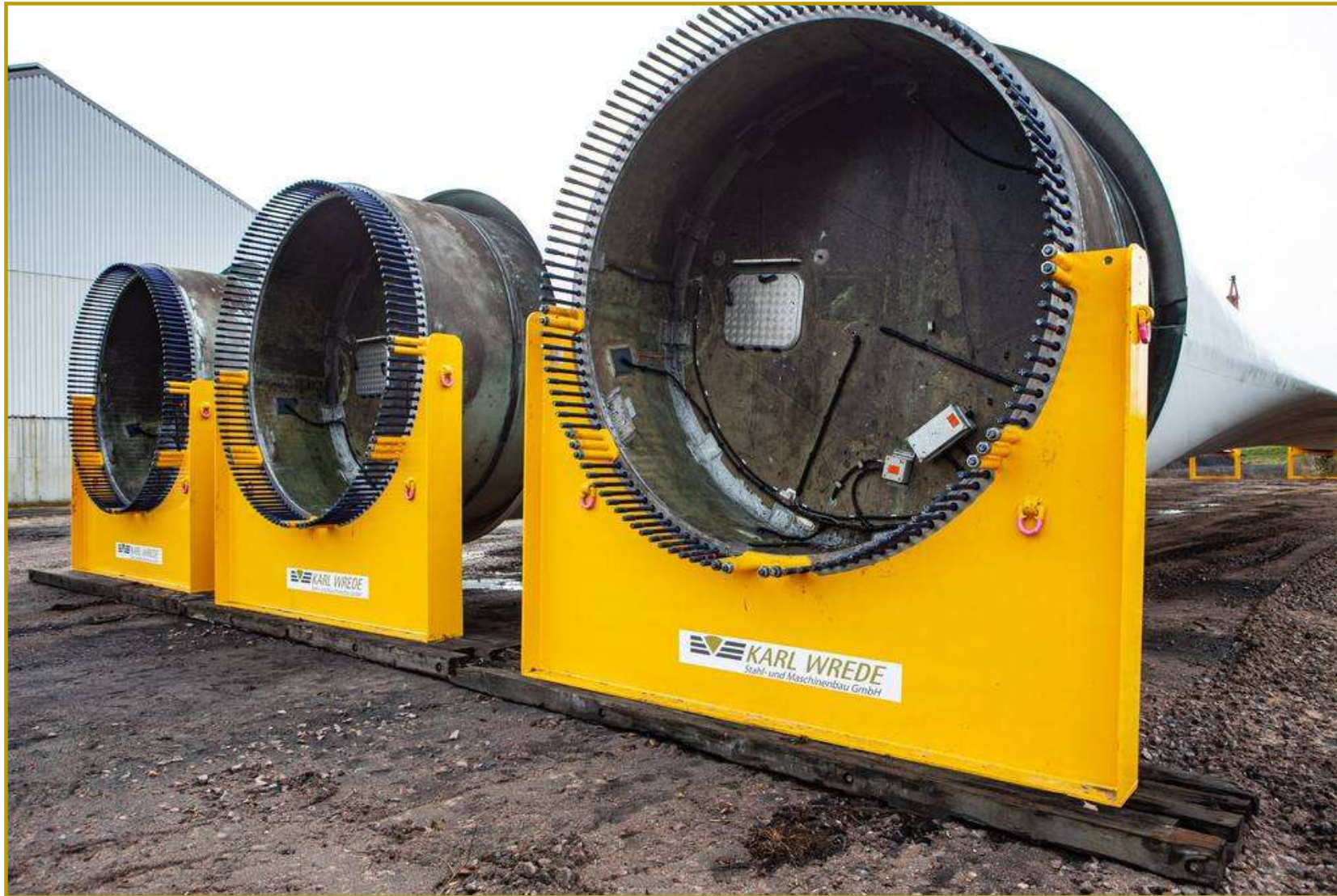
Rotor blade transport rack 5/6 MW
