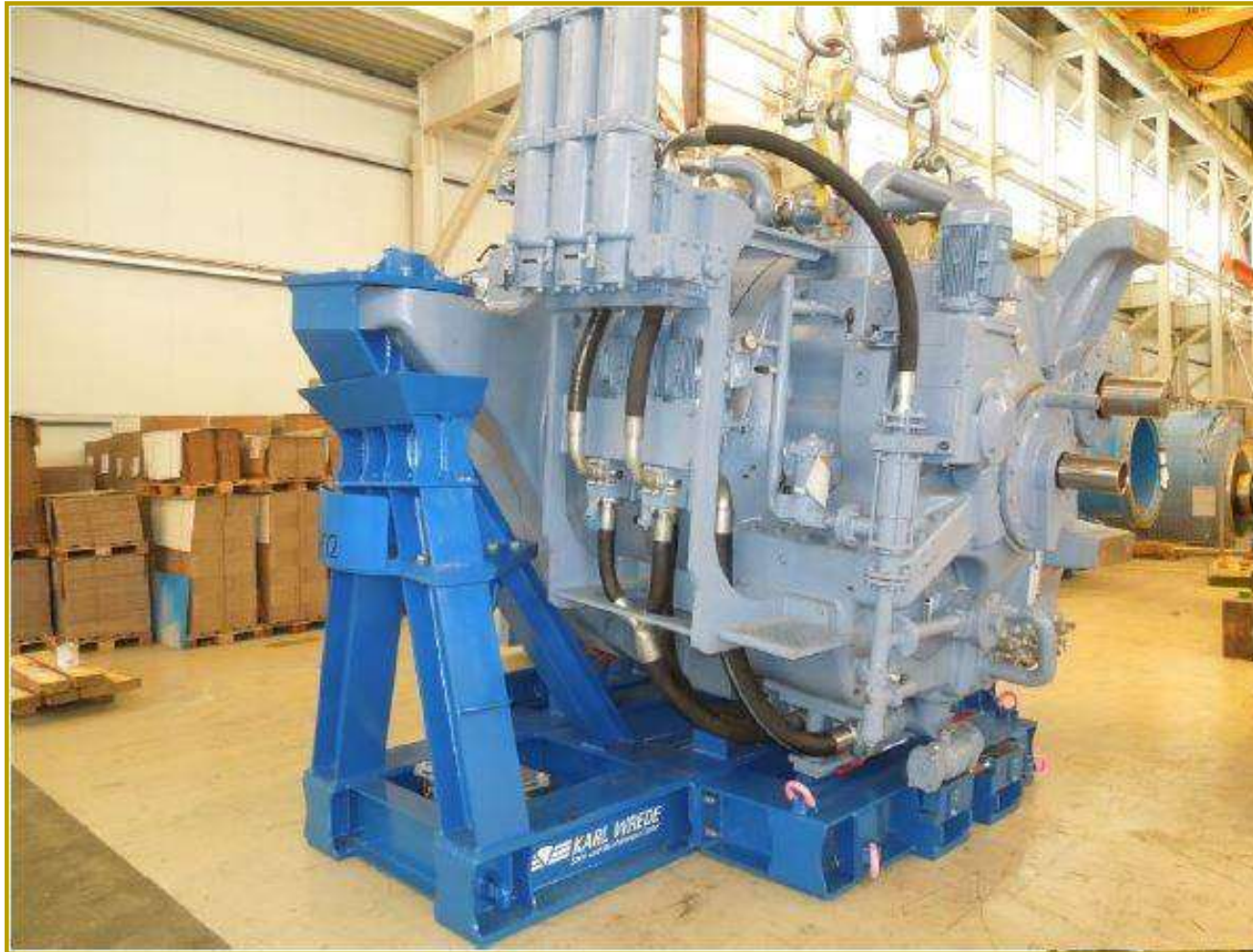
Offshore transport rack for gearbox 6 MW
