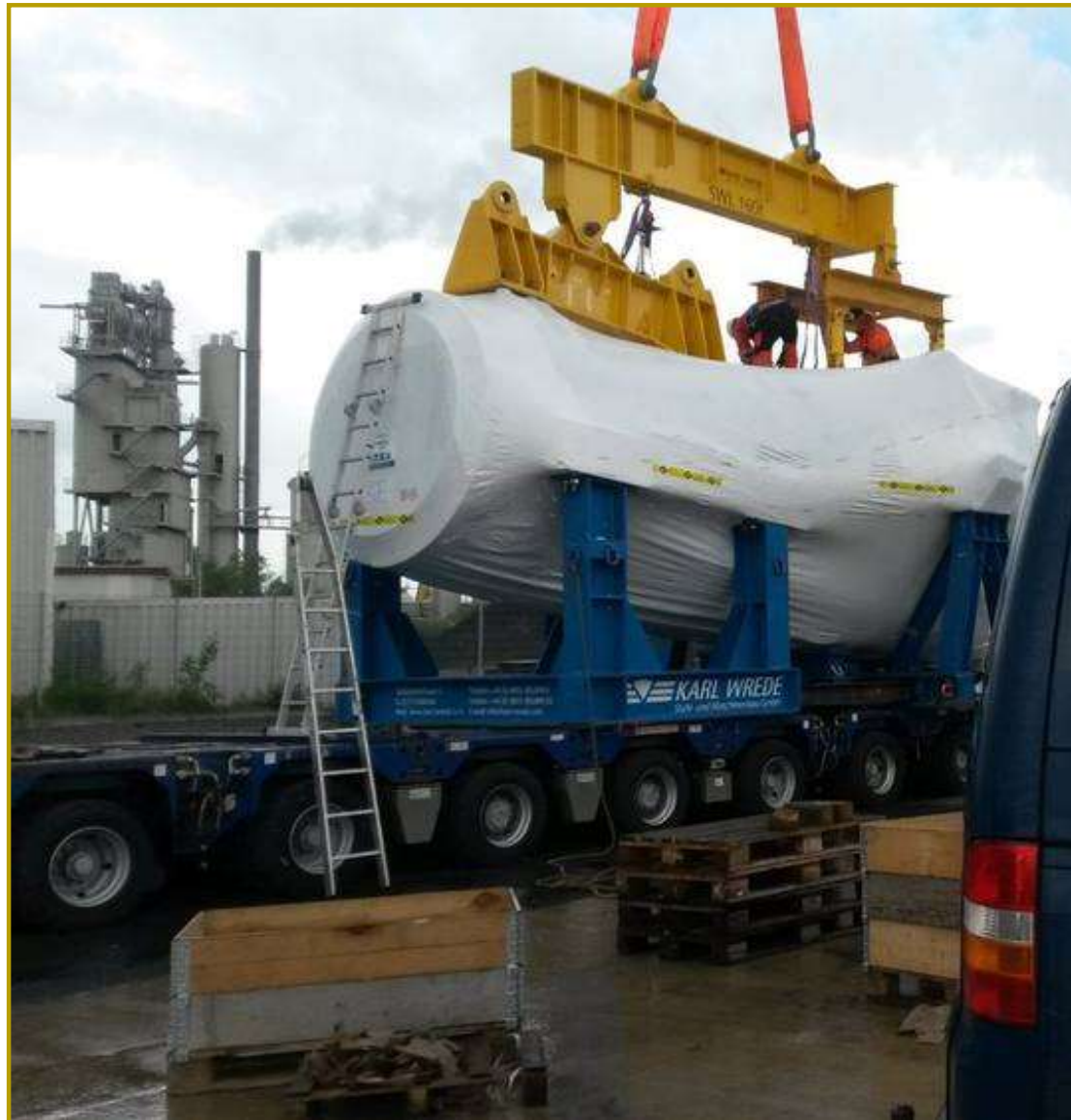
Lifting beam combination for drivetrain 6 MW
