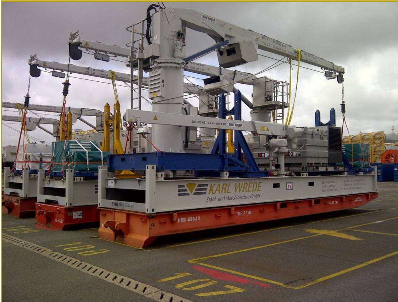
modified 40ft flatracks for component transport
