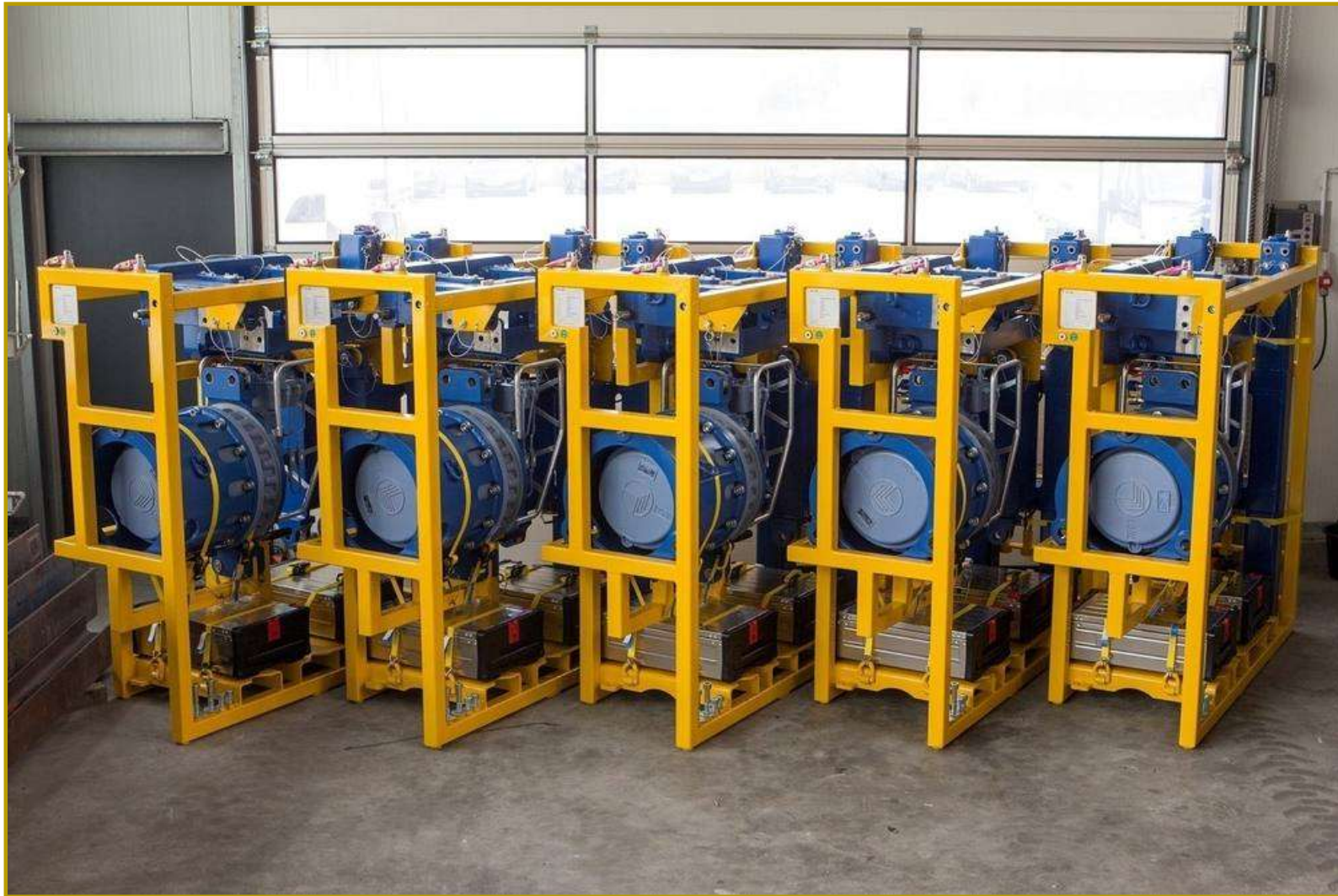
Hydraulic rotary drive system for drivetrain 6 MW offshore (single blade installation): delivery
