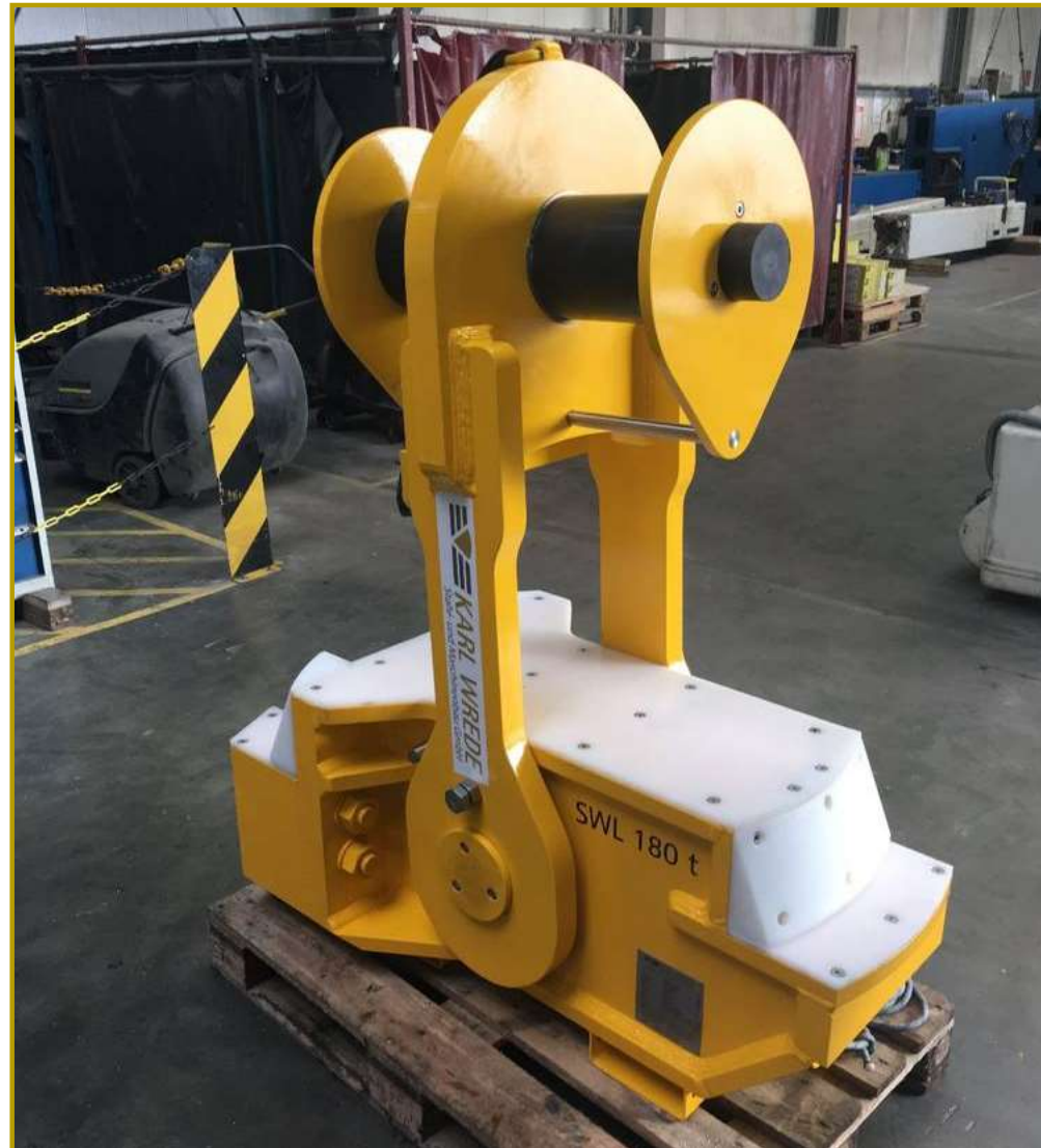
Lifting device for rotor star SWL 180 t – 6 MW
