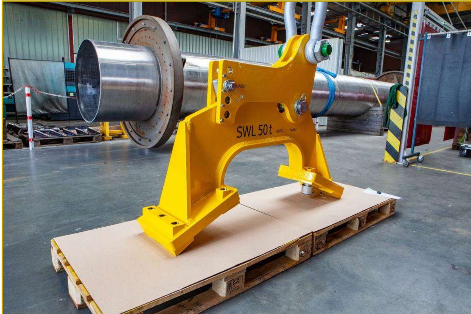
Rotor star lifting beam 2.3 MW – SWL 50 t
