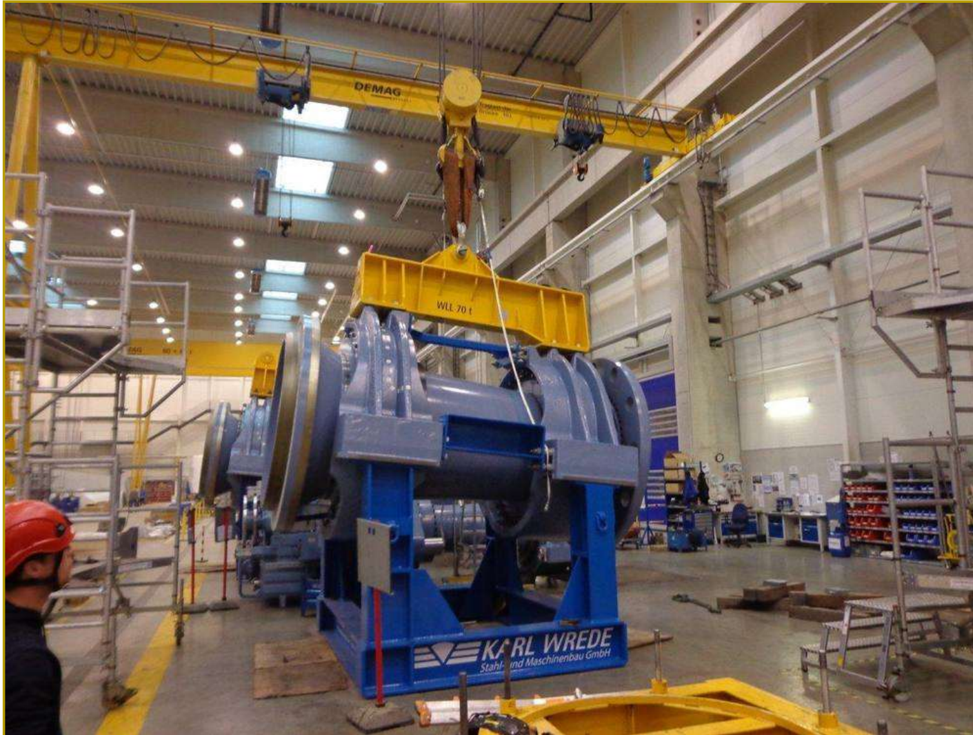
Rotor shaft assembly transport frame and lifting beam 5/6 MW
