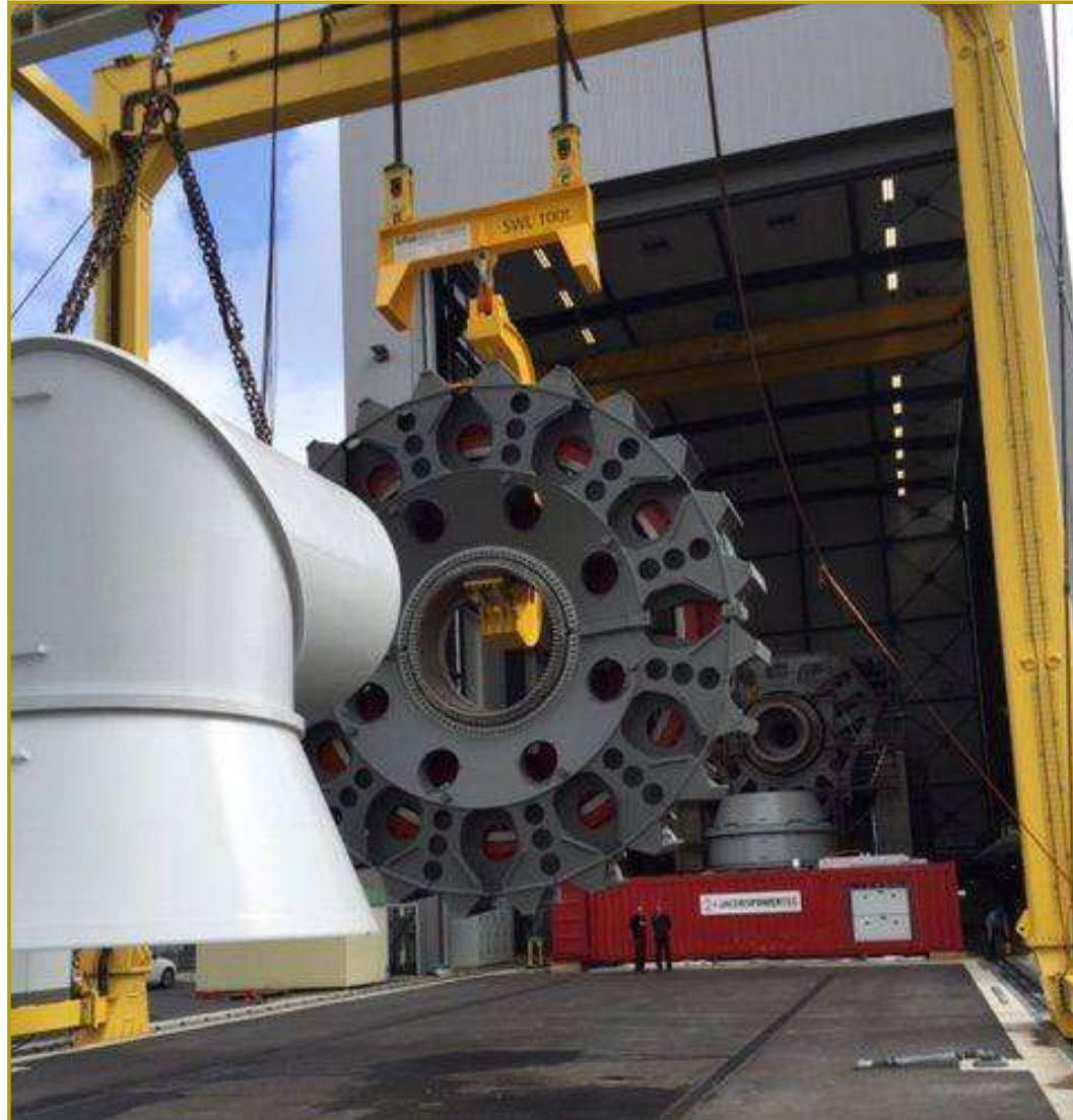
Coupling beam for generator 100 t
