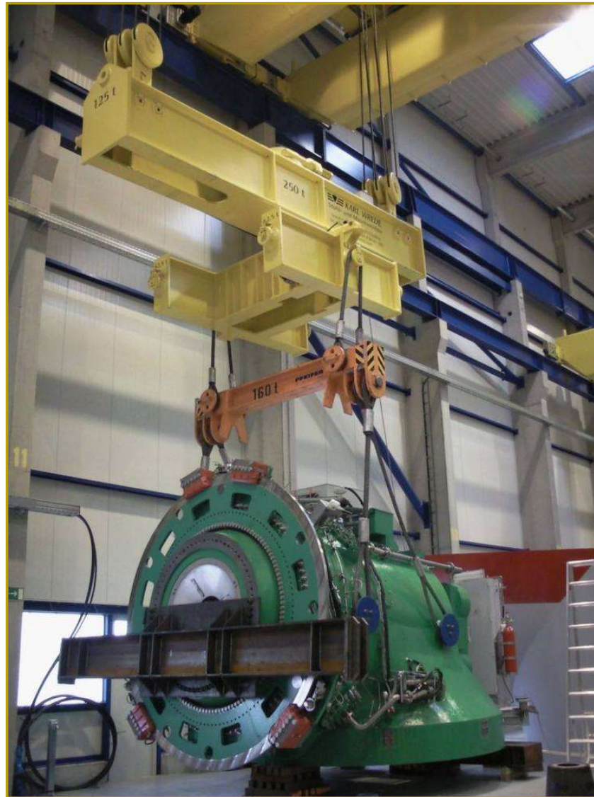
250 t assembly lifting beam combination
