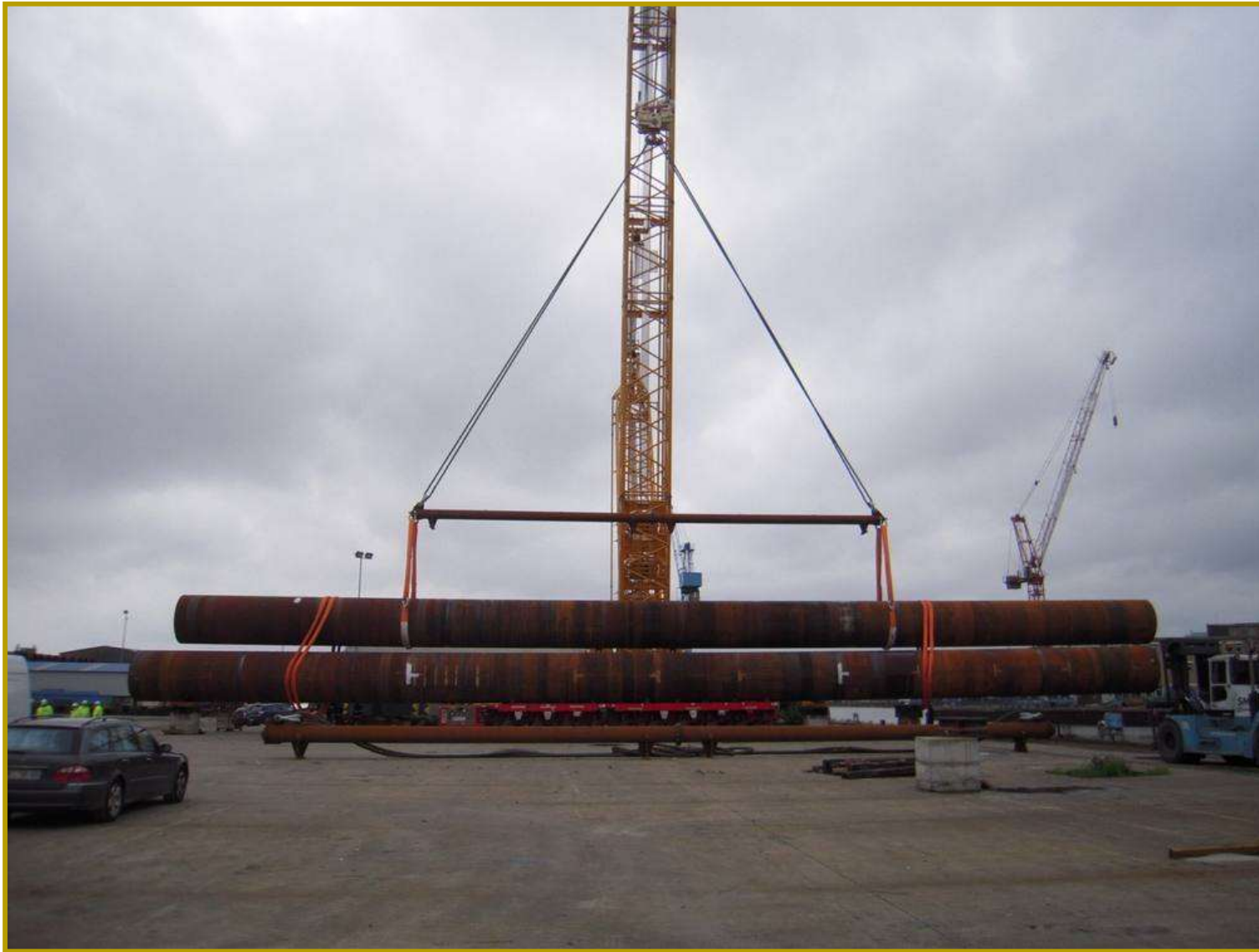
Pile lifting tool – SWL 270 t – l=25 m
