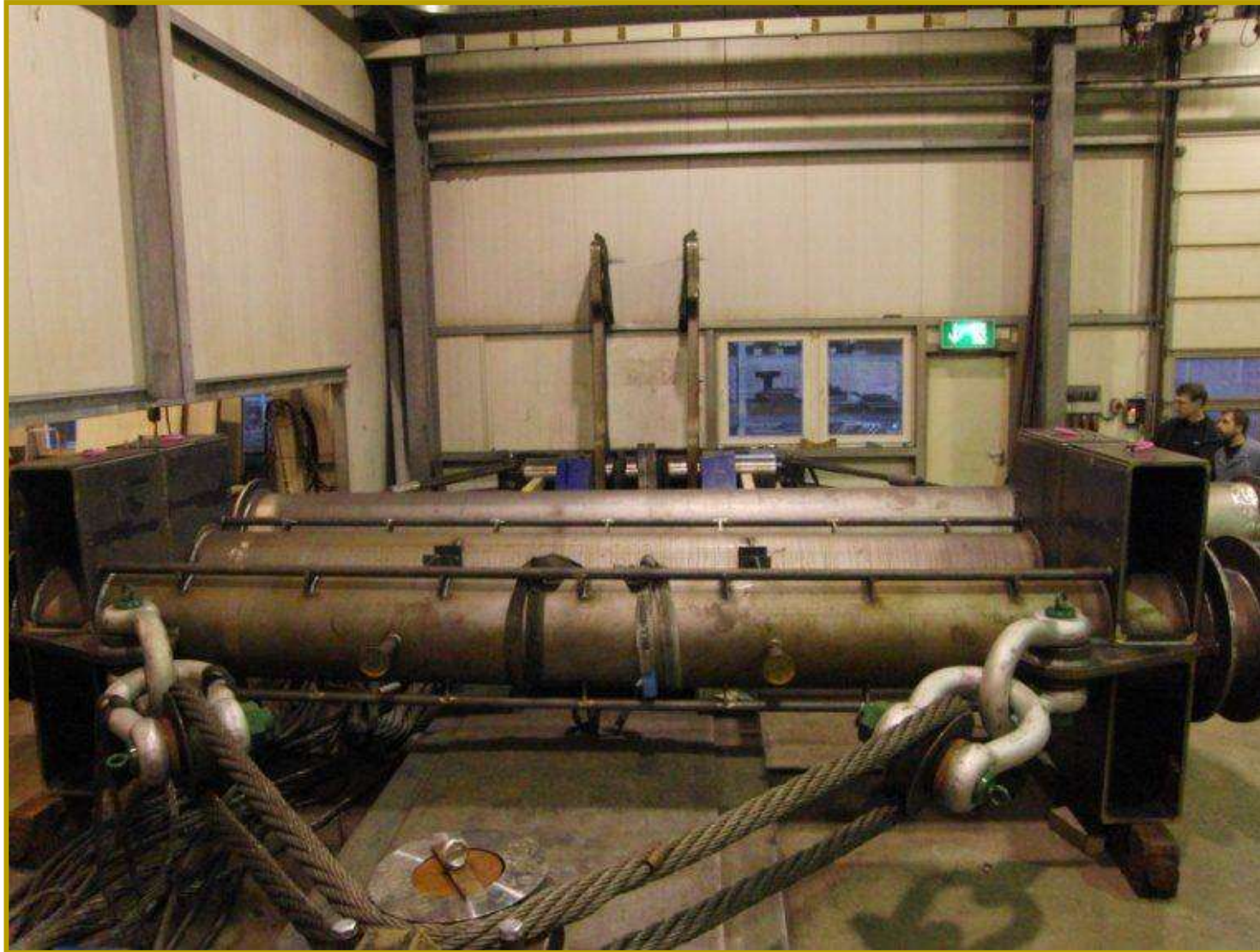
Upper lifting beam for tower – SWL 180 t
