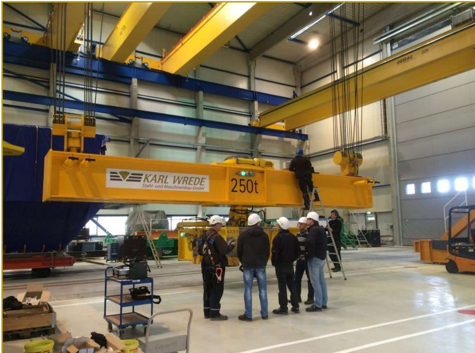
Assembly lifting beam 250 t with rotatable H-beam and hydraulic centre of gravity adjustment
