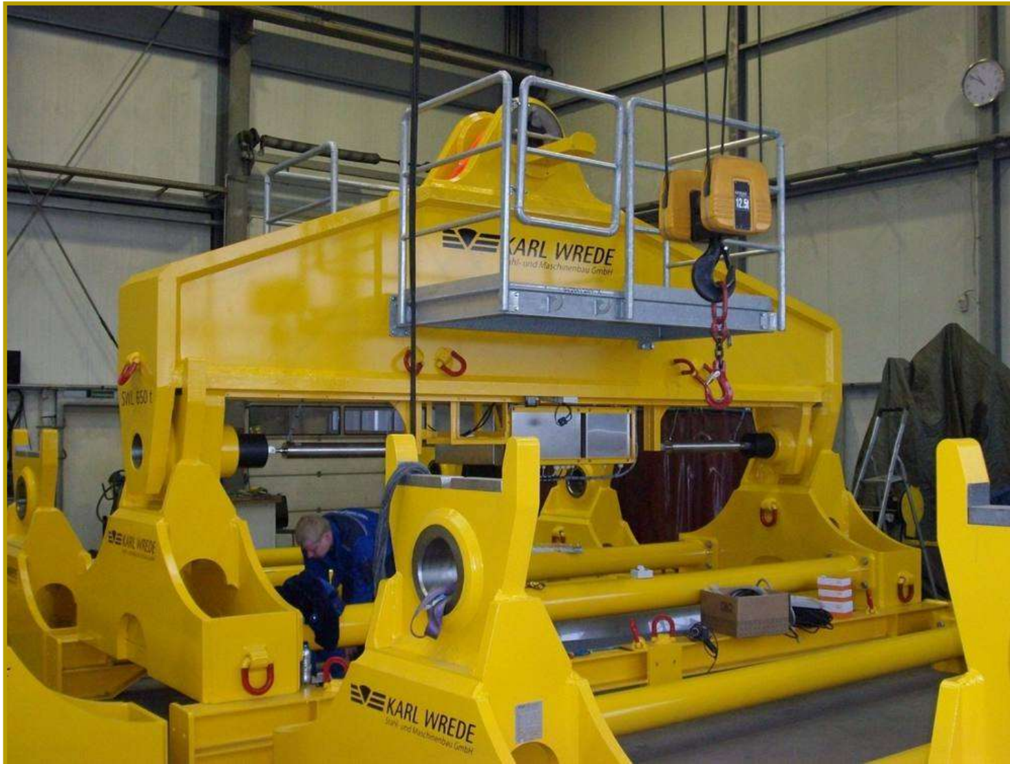
radio-remote-controlled installation beam SWL 650 t
