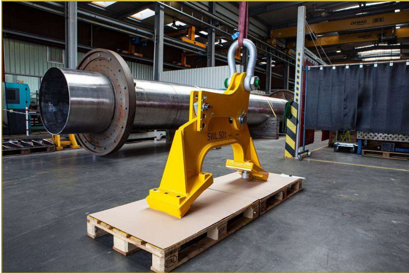
Rotor star lifting beam SWL 50 t
