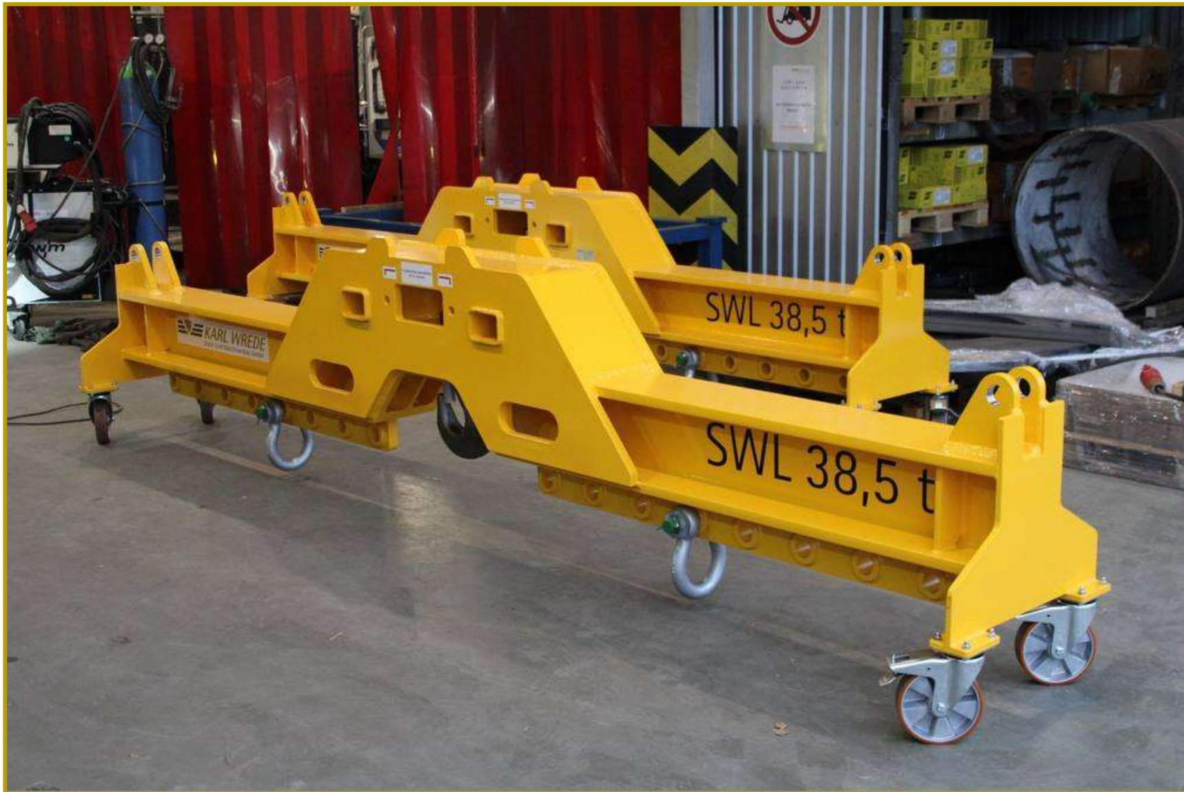
Special lifting beams SWL 38.5 t
