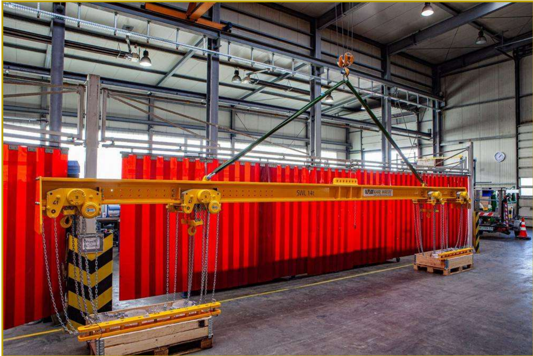
Special lifting beam for transformer replacement
