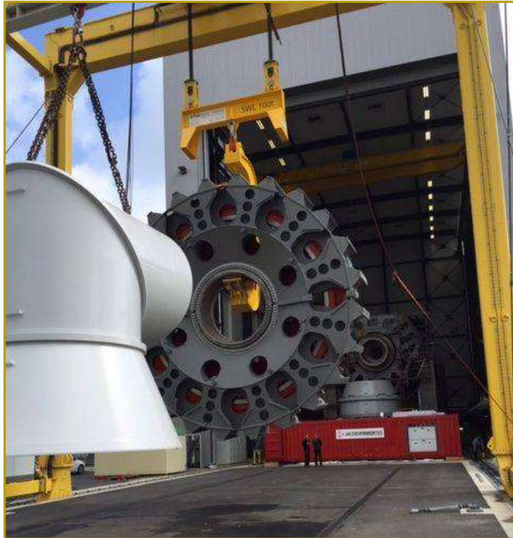
Lifting beam for rotor 100 t
