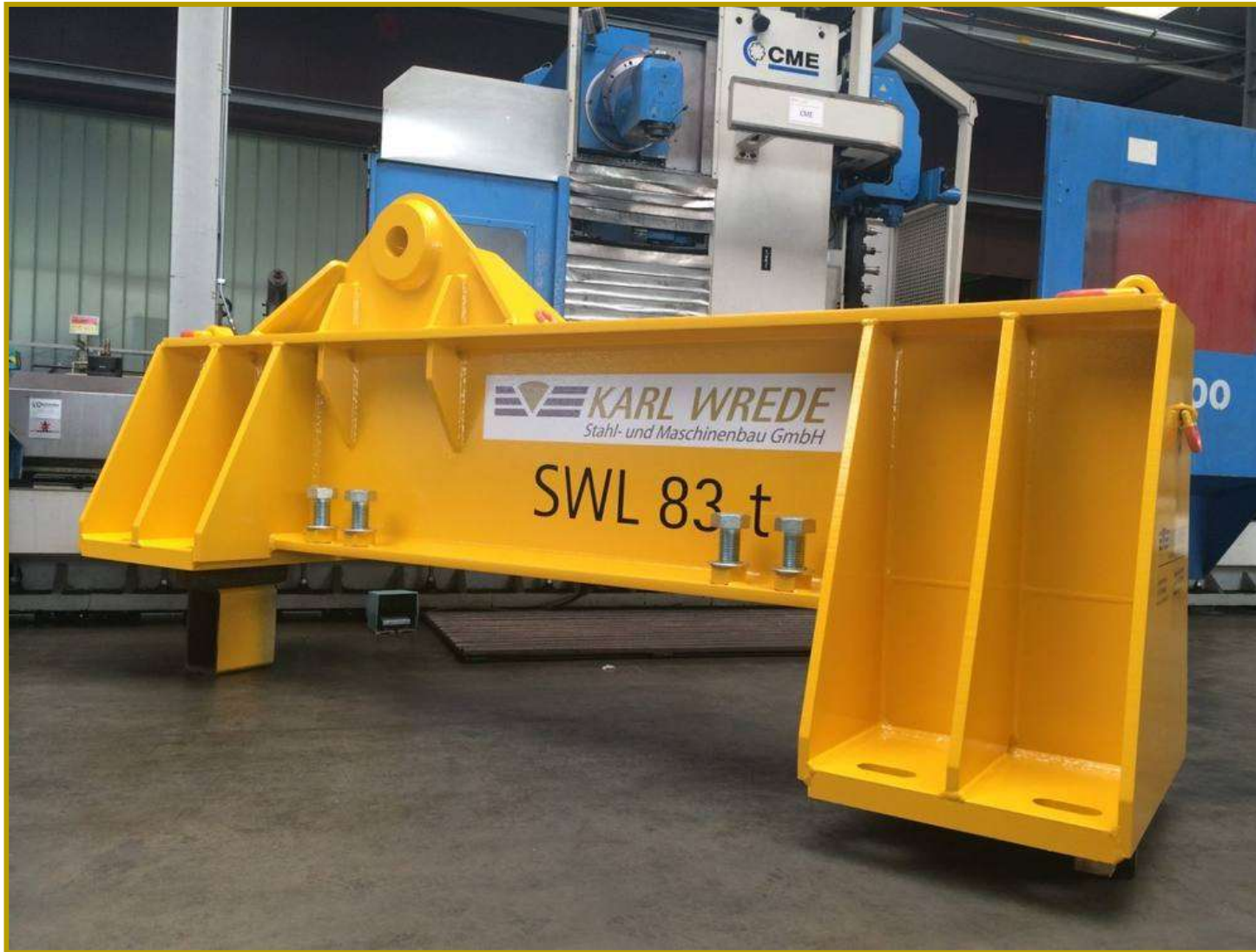
Drivetrain lifting beam SWL 83 t
