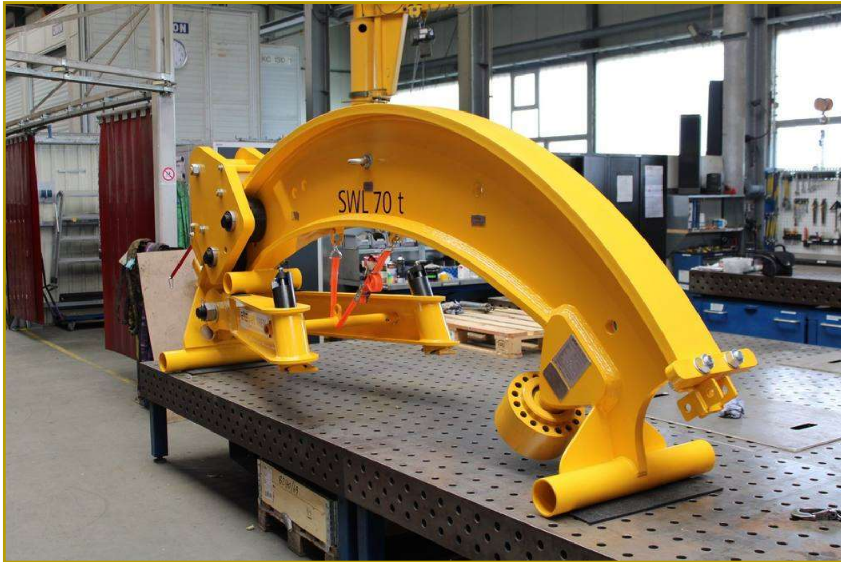
Rotor star lifting beam SWL 70 t
