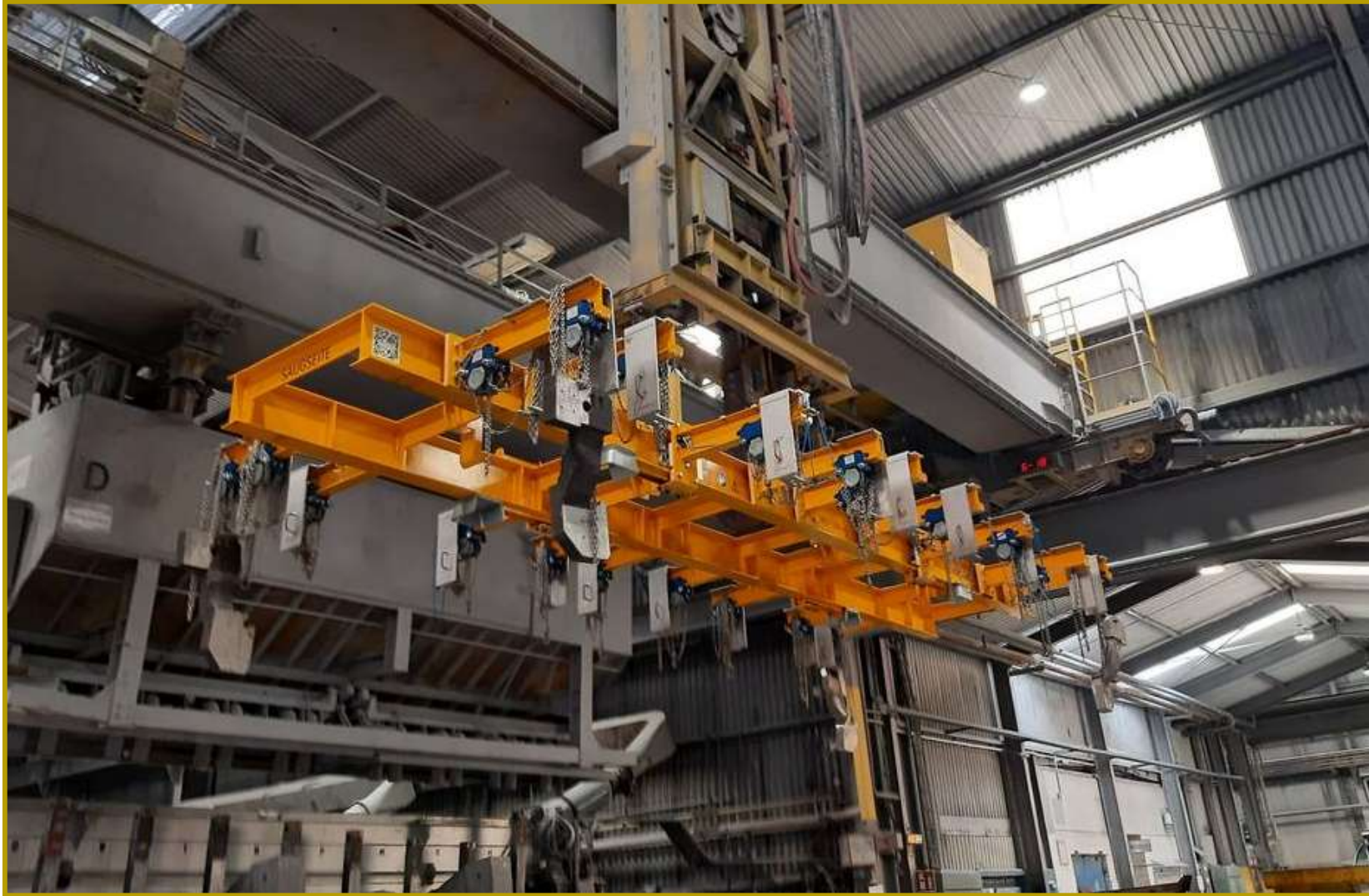
Approach lifting beam SWL 1.5 t
