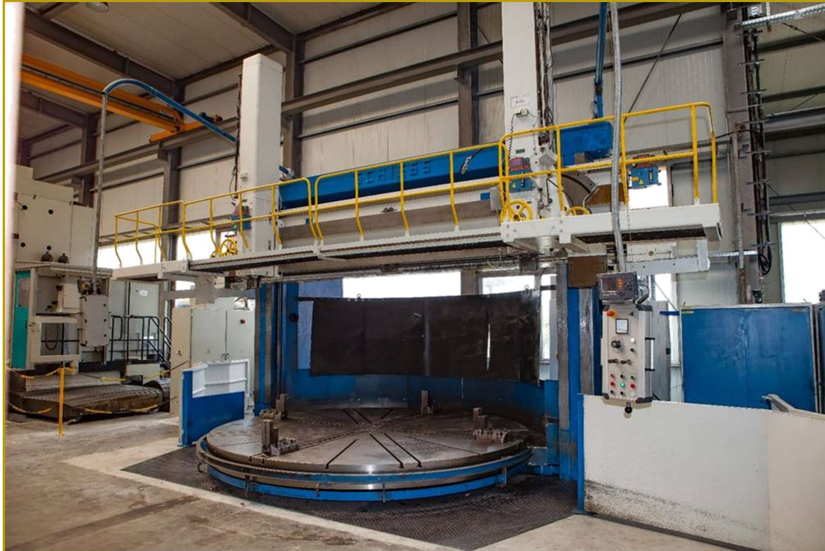
Vertical turning lathe Schless KZ 400-450 up to turning diameter 4,500 mm
