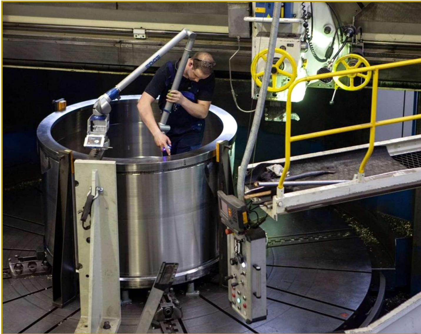
Dimensional inspection with FARO measuring arm
