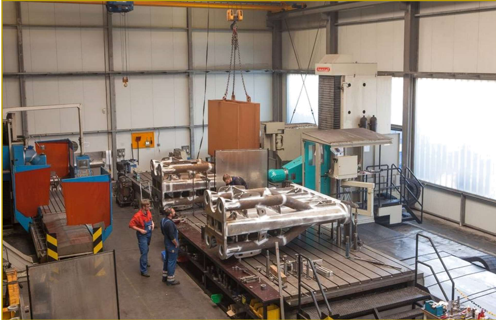
Assembly for offshore cable layer
