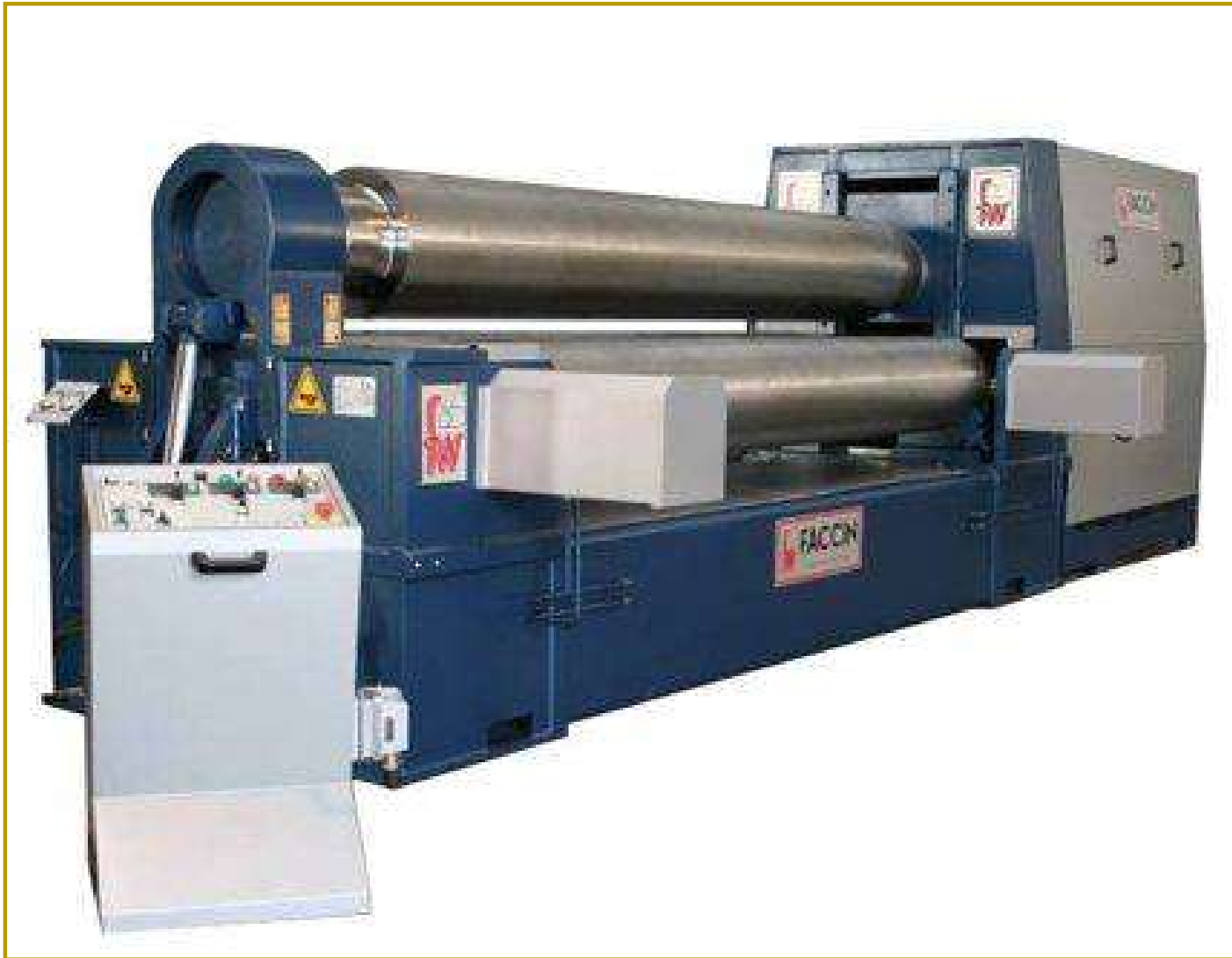
3-roll plate rolling machine FACCIN HAV 3145
