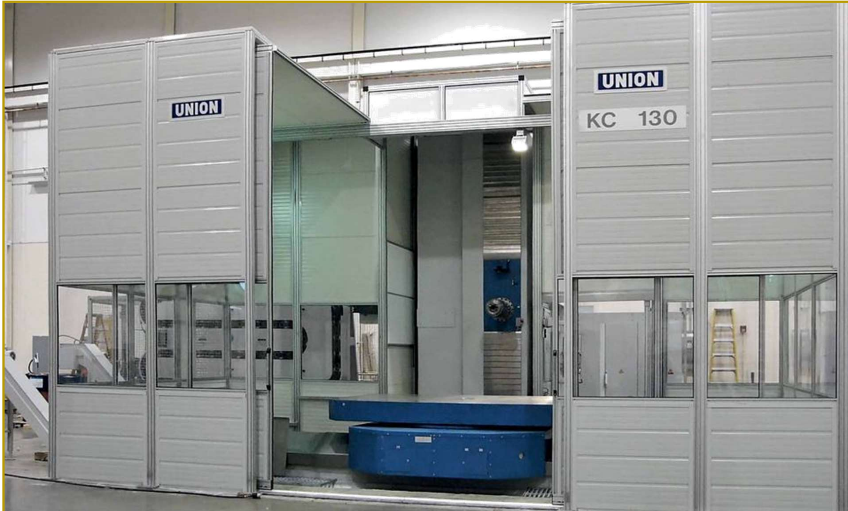
CNC table-type boring mill UNION KC 130/1 x/y/z/w: 3,200/2,500/1,500/800 mm, max. table load 8,000 kg
