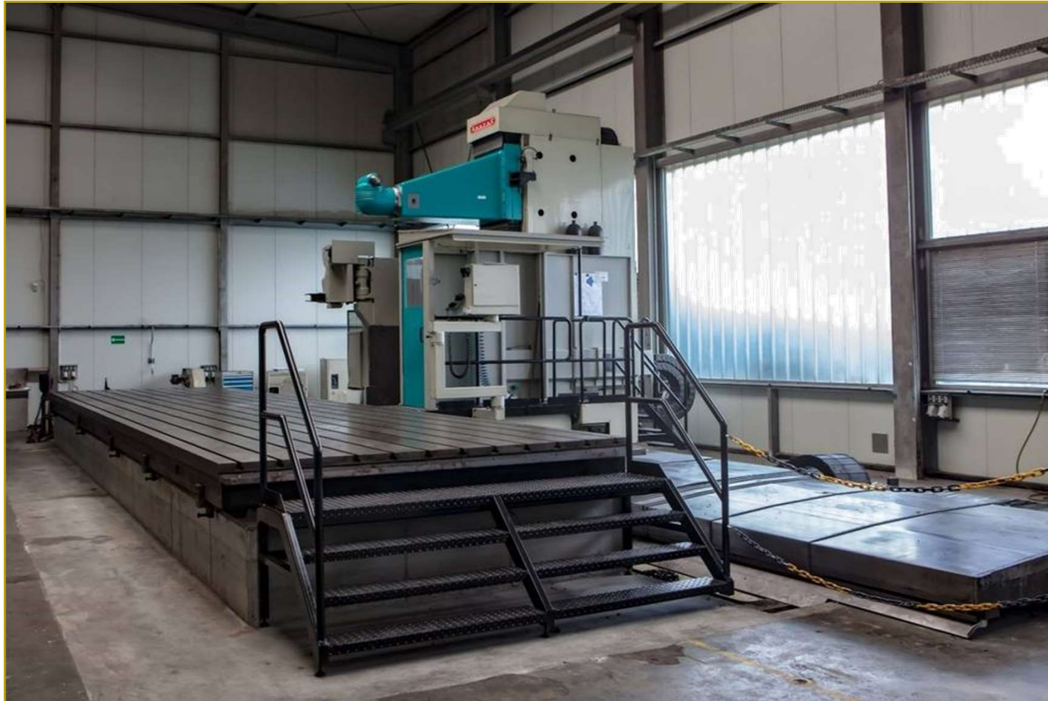
CNC travelling column milling machine Anayak HVM 12000 x/y/z: 11,300/2,000/2,400 – 25 t unit weight
