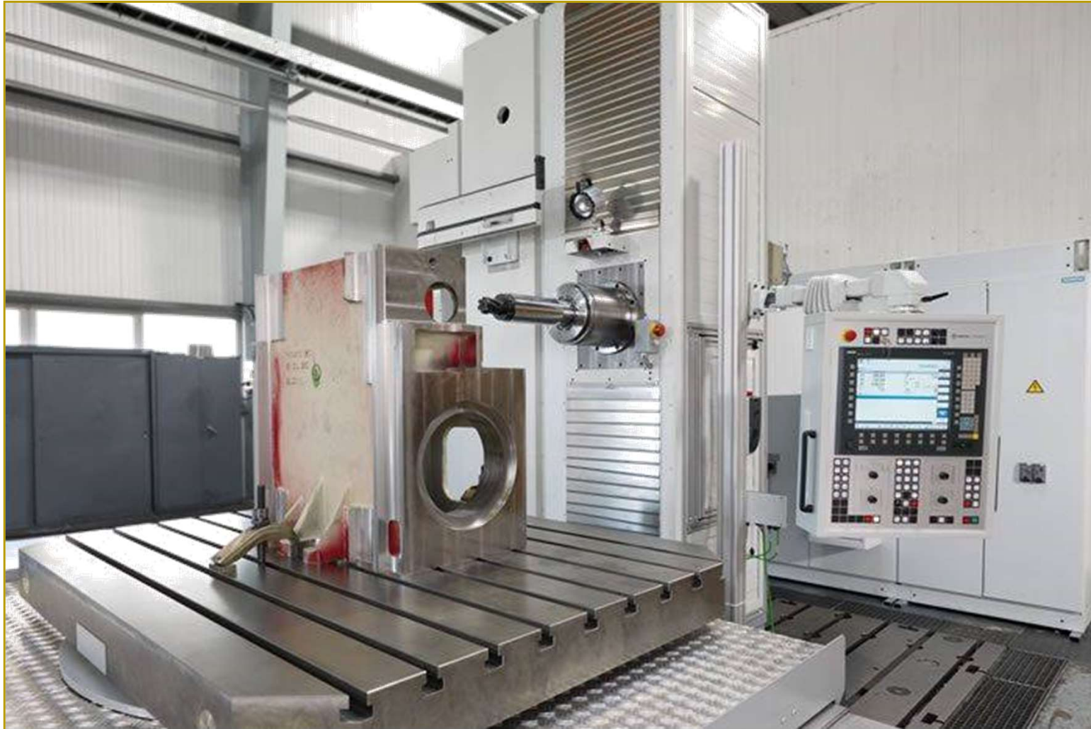
CNC table-type boring mill UNION TC 110 with pallet changer x/y/z/w: 1,500/2,000/1,600/550 mm, max. table load 4,000 kg
