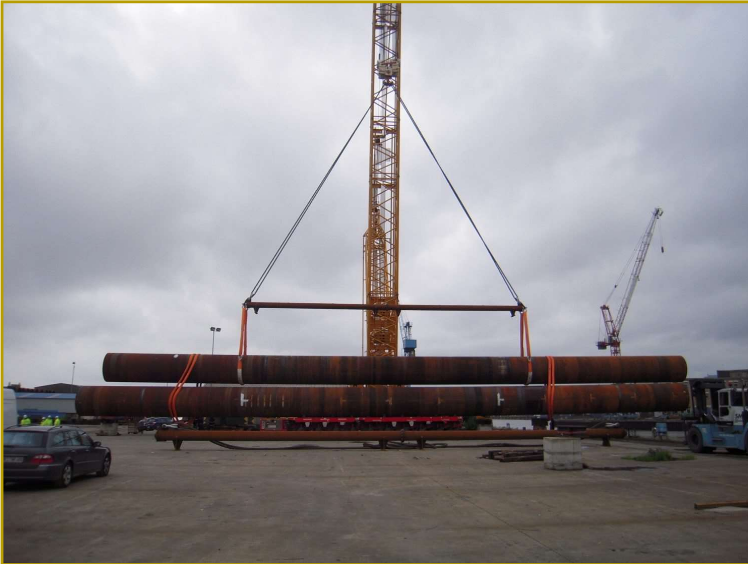
Pile lifting tool – SWL 270 t – l=25 m
