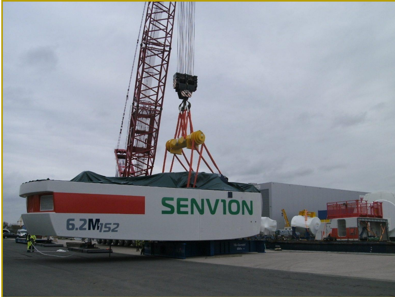
Nacelle lifting beam - SWL 480 t
