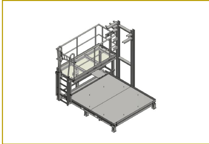
Custom support frame for vessel
