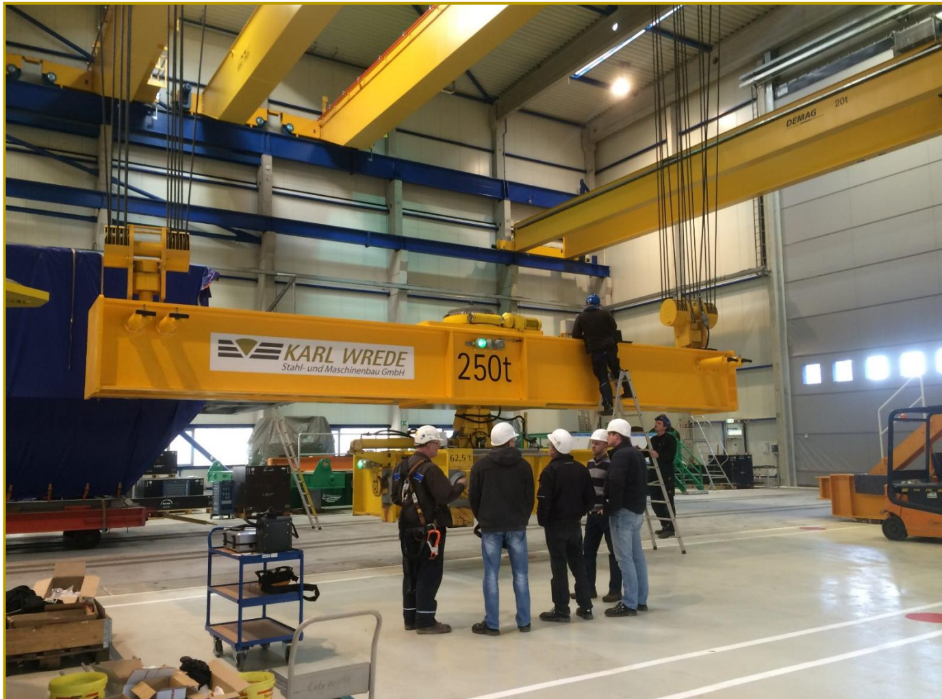
250 t installation lifting beam with rotating H-beam and hydraulic centre-of-gravity adjustment
