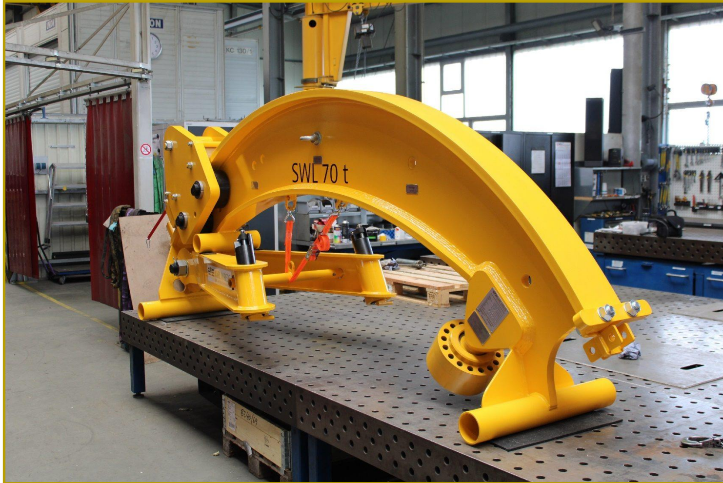
Rotor star lifting beam - SWL 70 t
