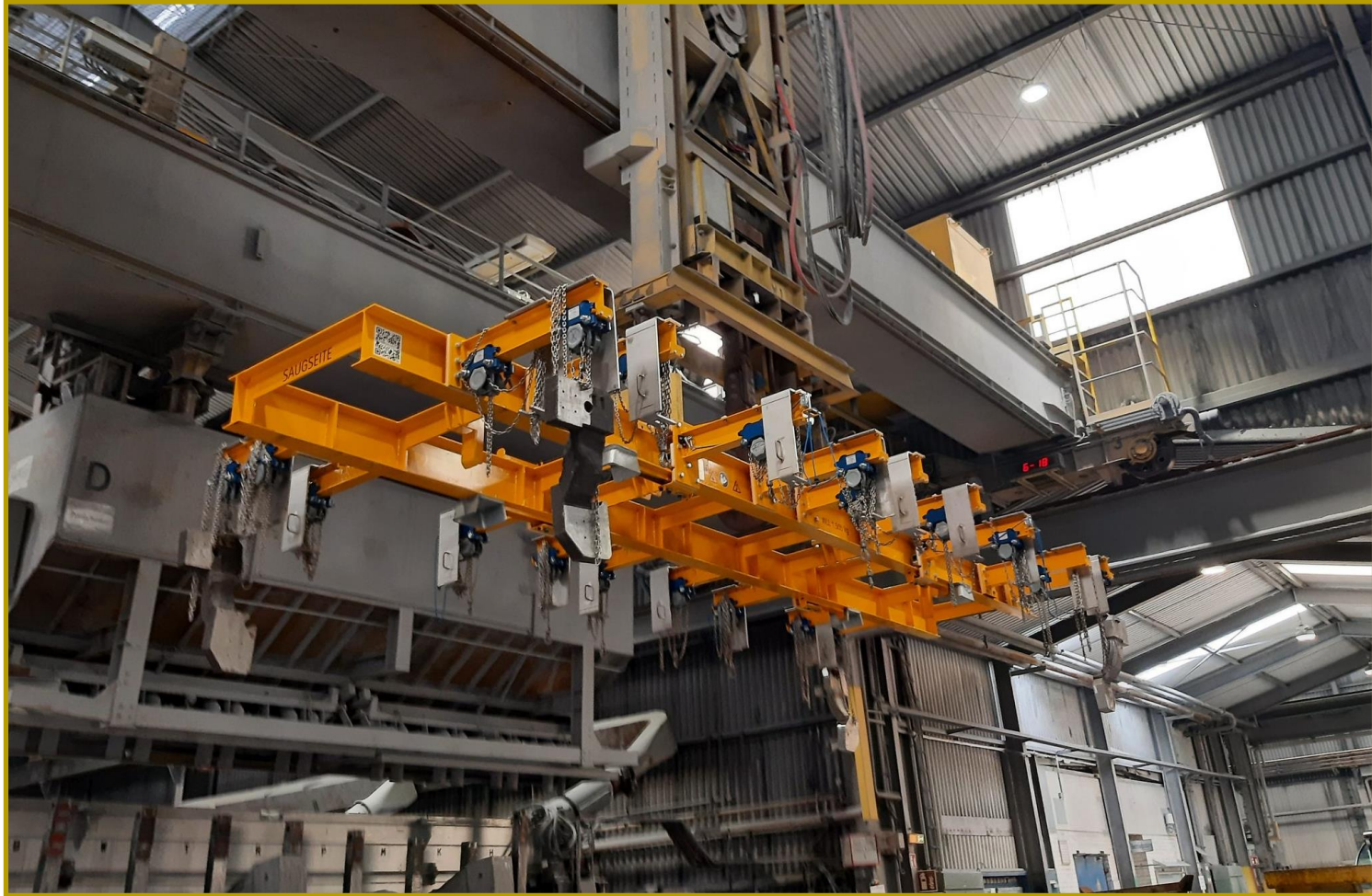
Positioning lifting beam - SWL 1.5 t
