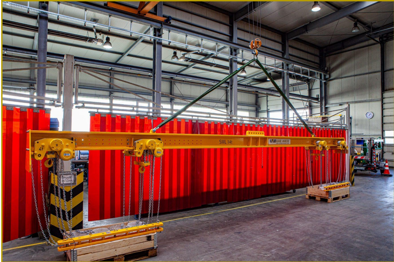
Custom lifting beam for transformer replacement
