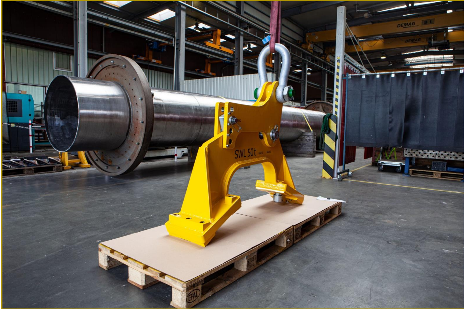
Rotor star lifting beam - SWL 50 t
