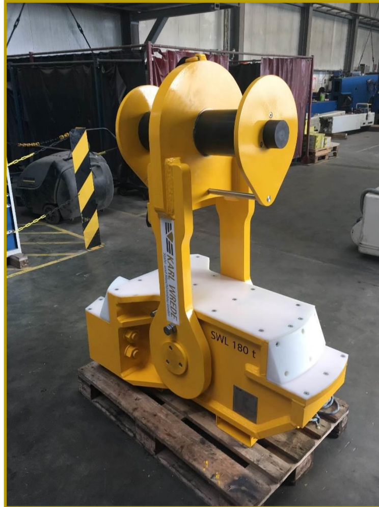
Rotor star lifting beam - SWL 180 t
