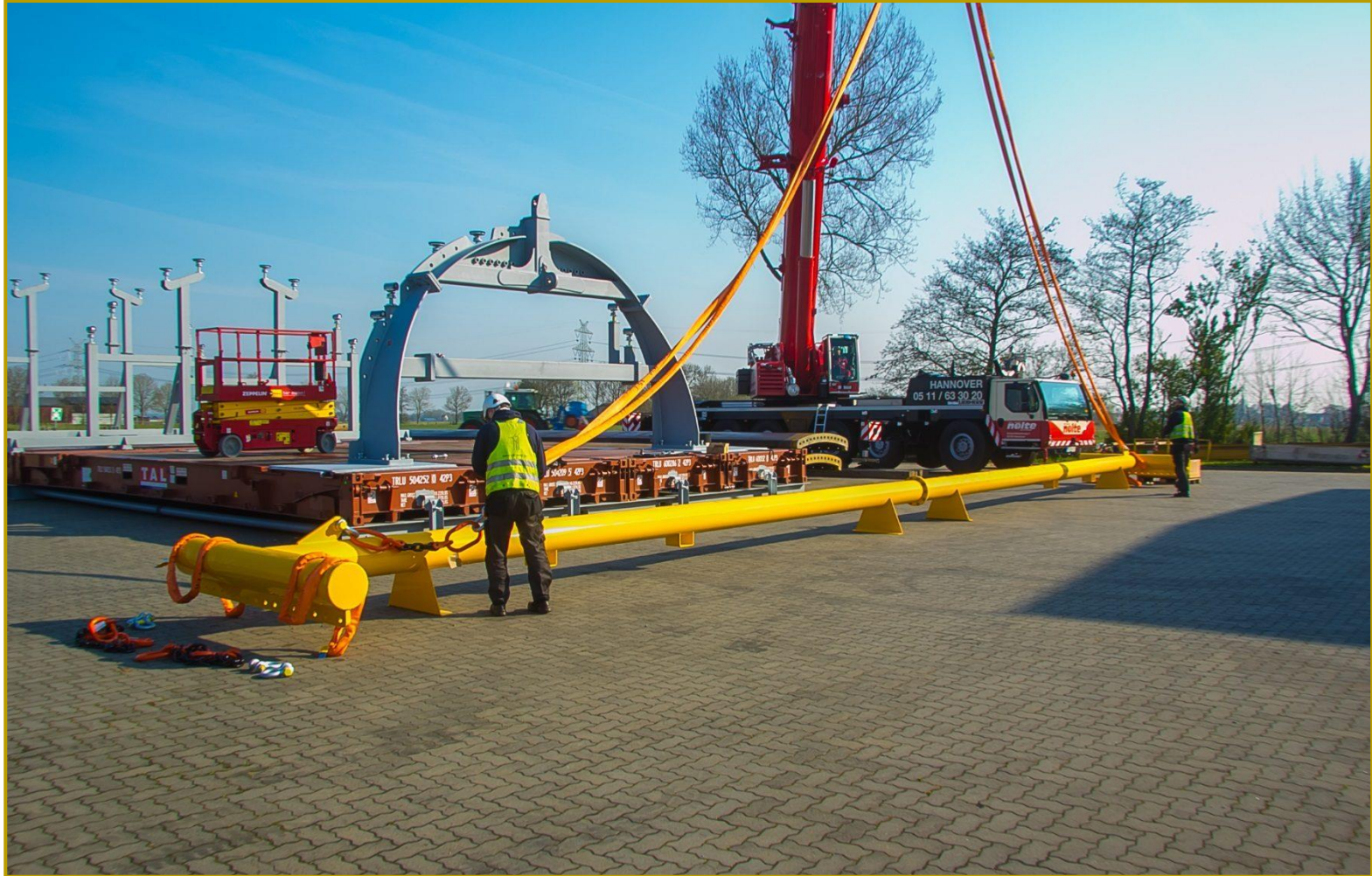
Spreader beam for segmented tubular steel towers
