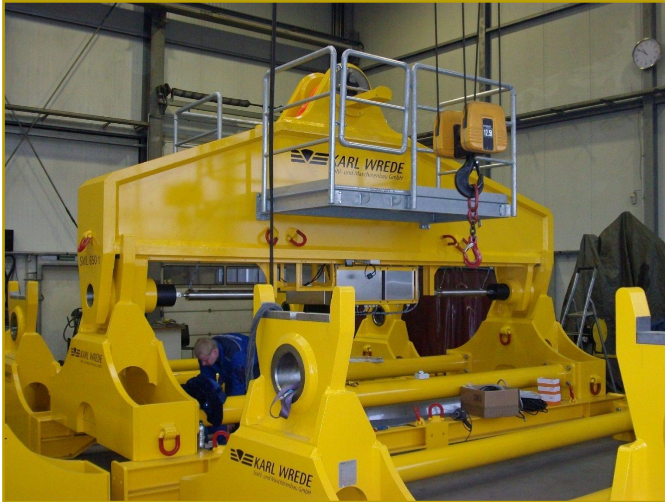
Remote-controlled installation lifting beam - SWL 650 t
