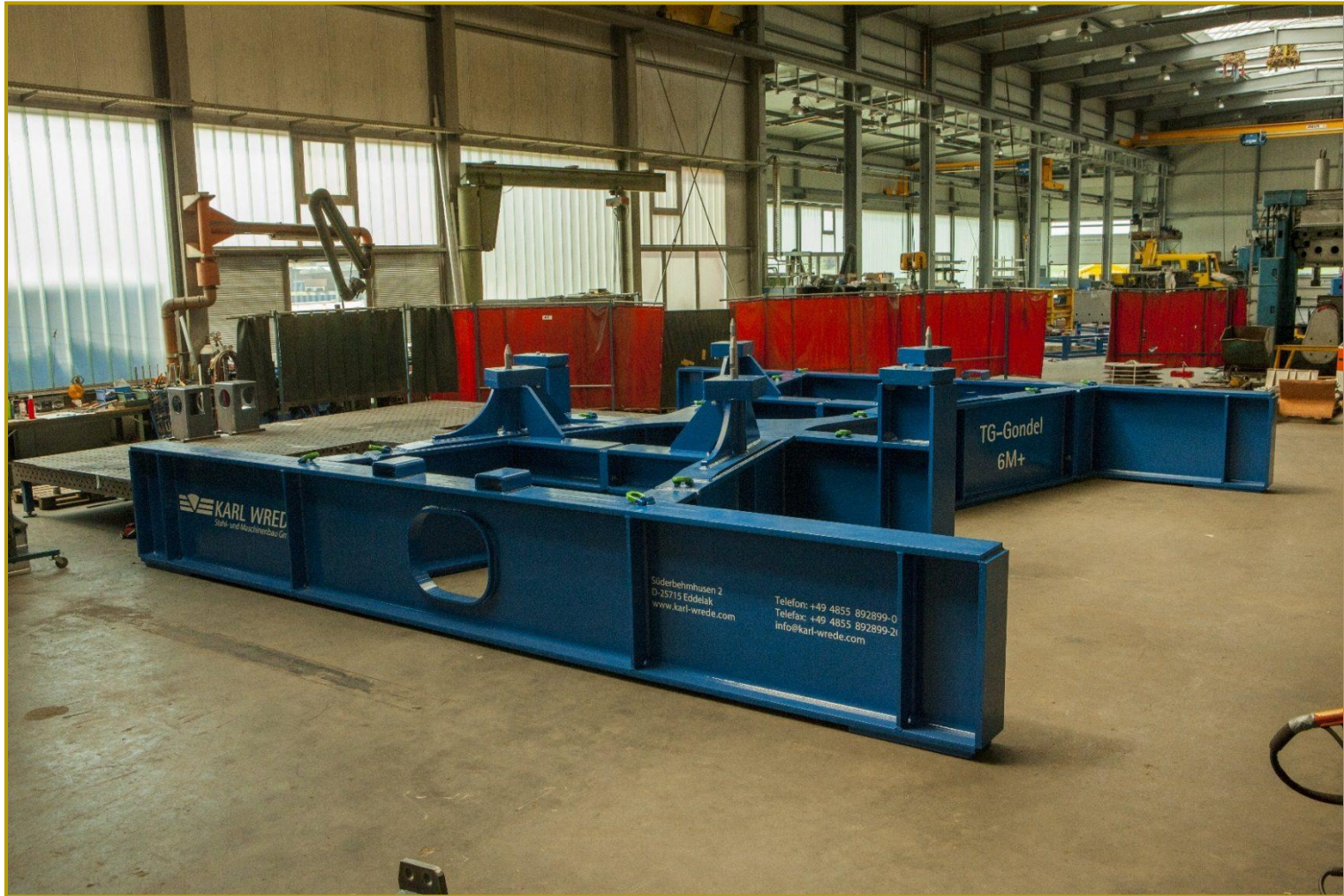
Wind turbine transport frame
