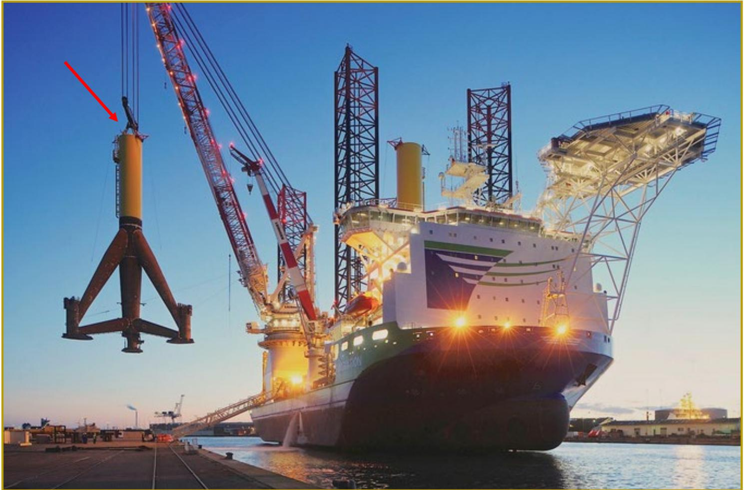
Tripod Lifting Tool SWL 950 t
