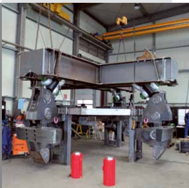
Load testing setup 950 t beam
